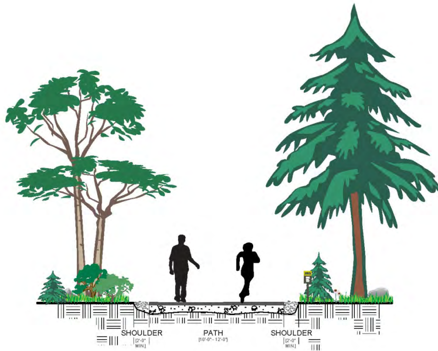
Figure 1 – Typical cross-section for a shared use path
