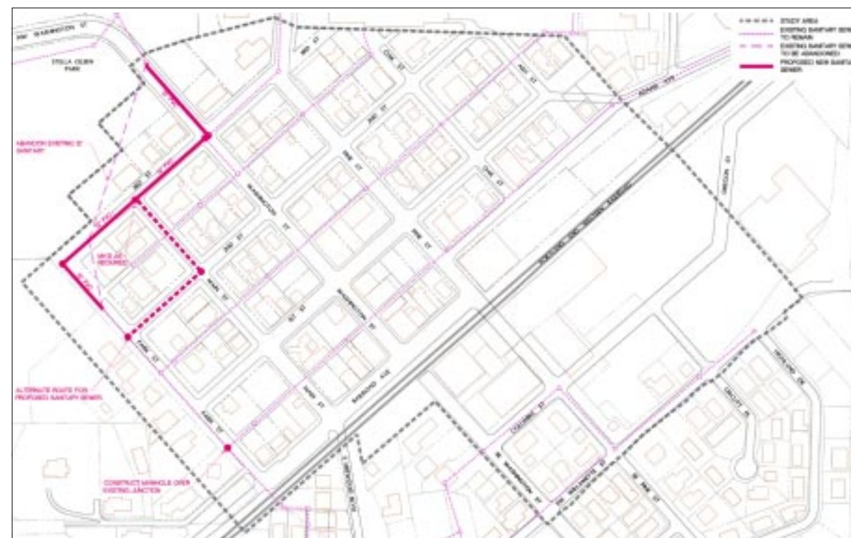
Sanitary sewer reconstruction/rehabilitation plan
