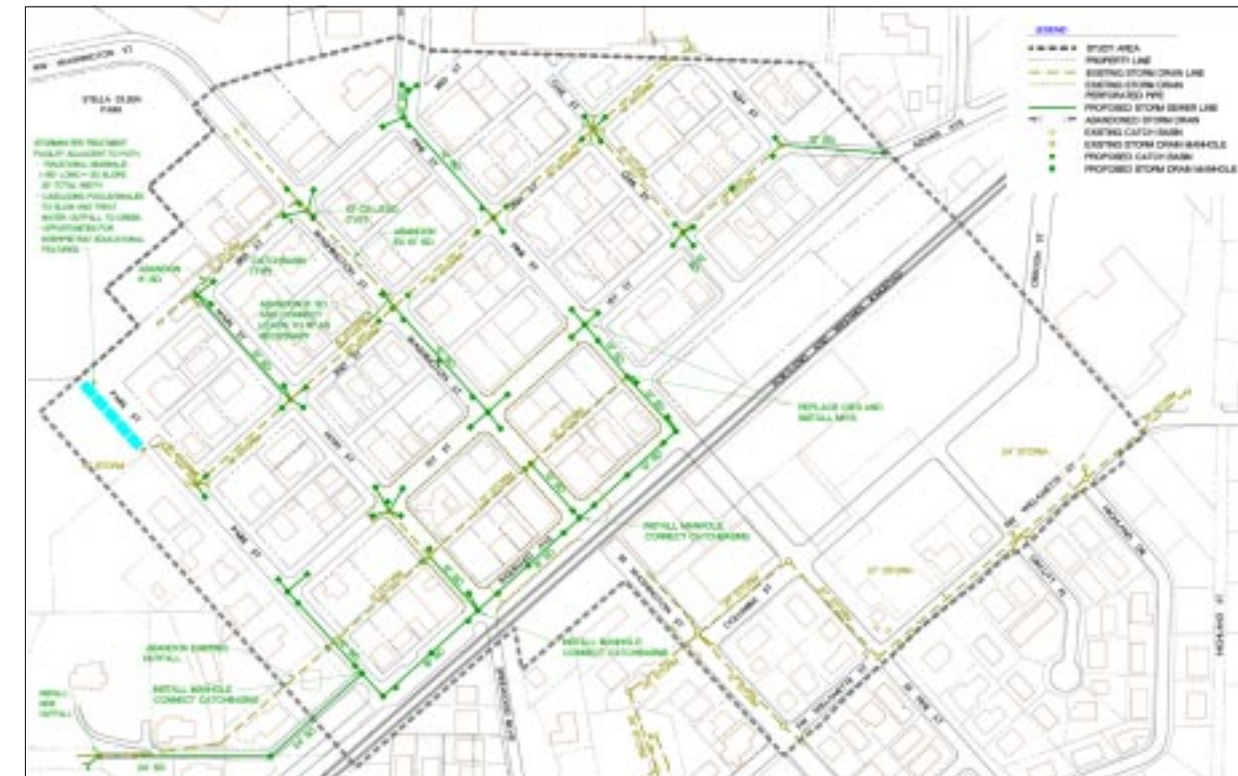
Storm sewer master plan
