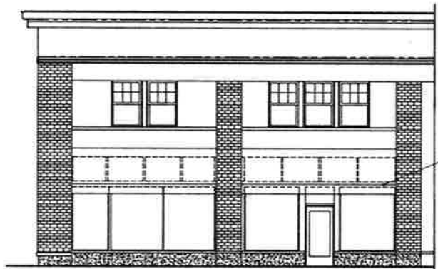
RAILROAD STREET ELEVATION: EXISTING SCALE: 1/4" = 1'-0"
