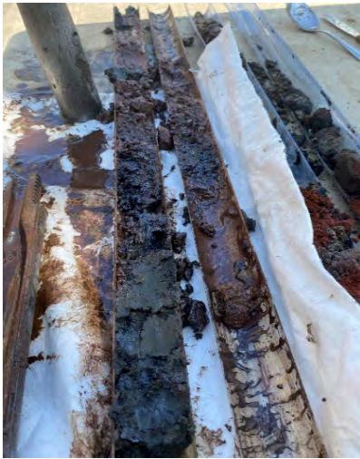
Photo 1: Contaminated Soil Core - B-14, NW 9th Ave between Kearney and Lovejoy
