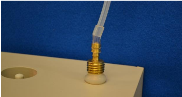
Figure 5. VAPOR PIN® sample connection
