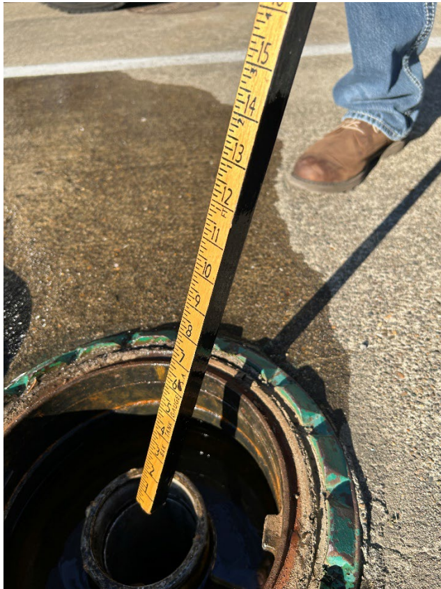
7: Stick gauging what fuel is in the tank
