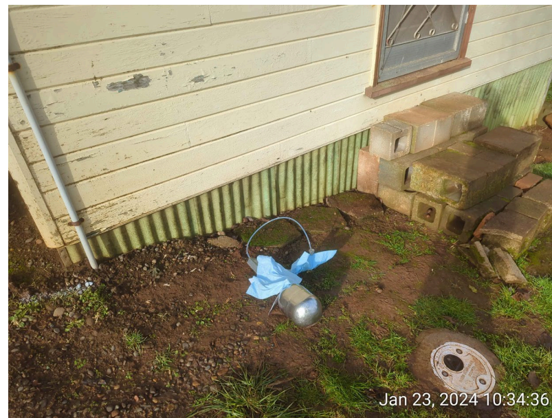
Typical soil gas sampling set up (note blue rags saturated with IPA for leak check)
