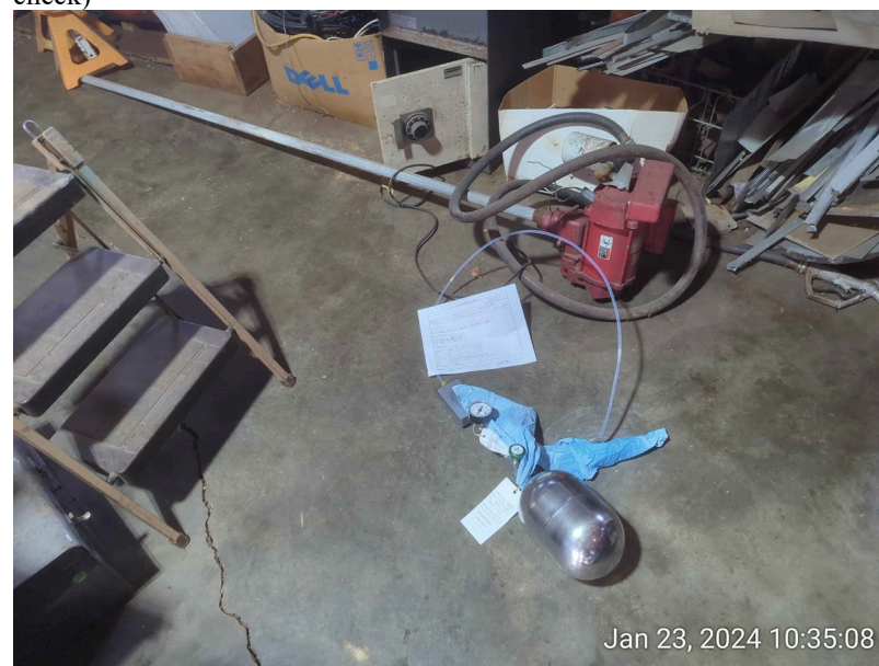
Typical sub-slab vapor sampling set up.
