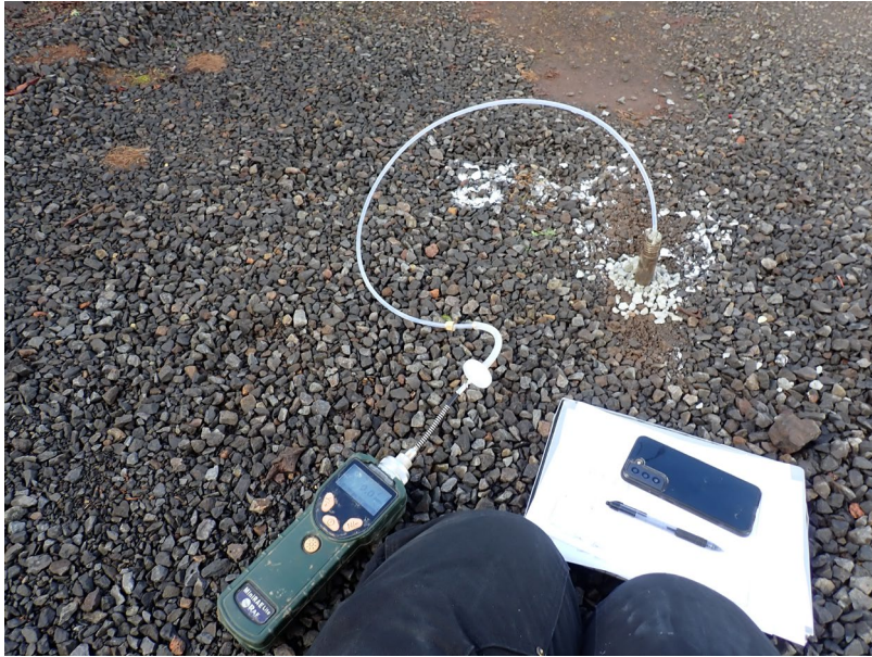
Purging and screening soil gas with PID
