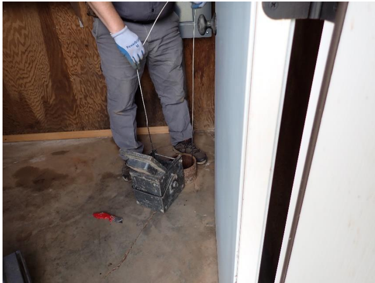
Determining depth to water and total depth in well
