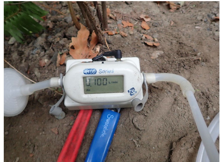
During sample collection, a digital rotameter was utilized to monitor and maintain a steady sample rate.
