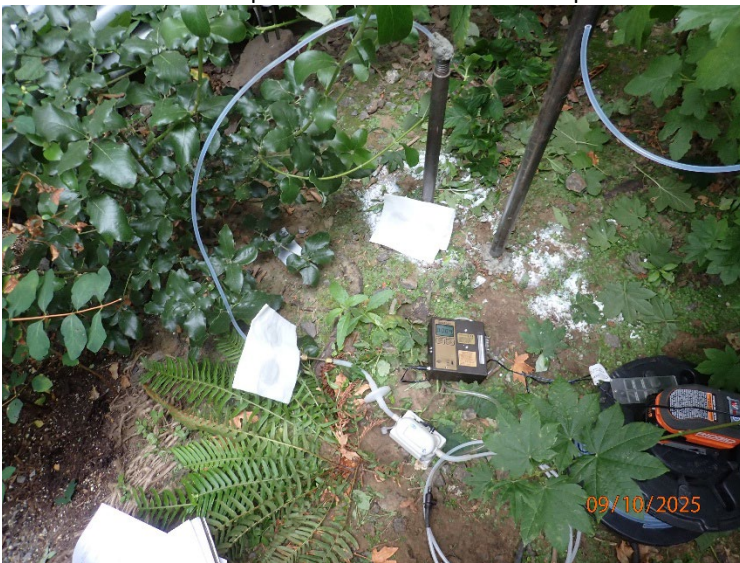
View of soil gas sample collection using EPA Method TO-17. Rags saturated with isopropyl alcohol were placed over sample train connections for leak detection.
