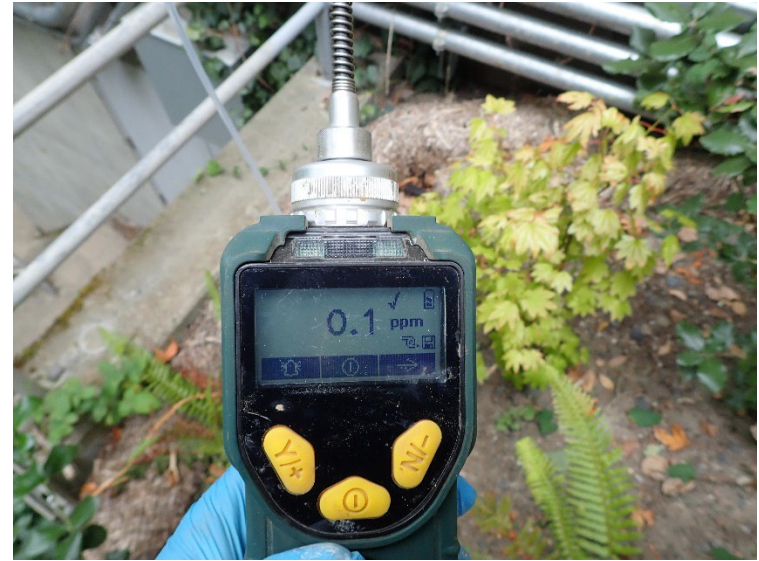
A photoionization detector (PID) was used to purge ambient air from the sample train and screen soil gas for volatile constituents.
