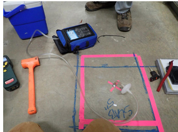
A landfill gas meter was utilized to measure concentrations of oxygen and other gases.
