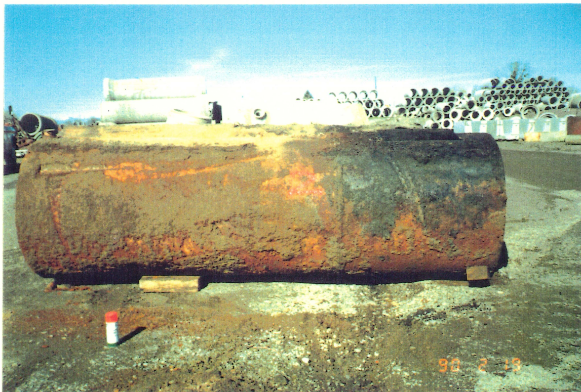
Figure 4: Hamrick site 1,000 gallon UST, labeled H-UST-2. The fill end of the UST is heavily stained.
