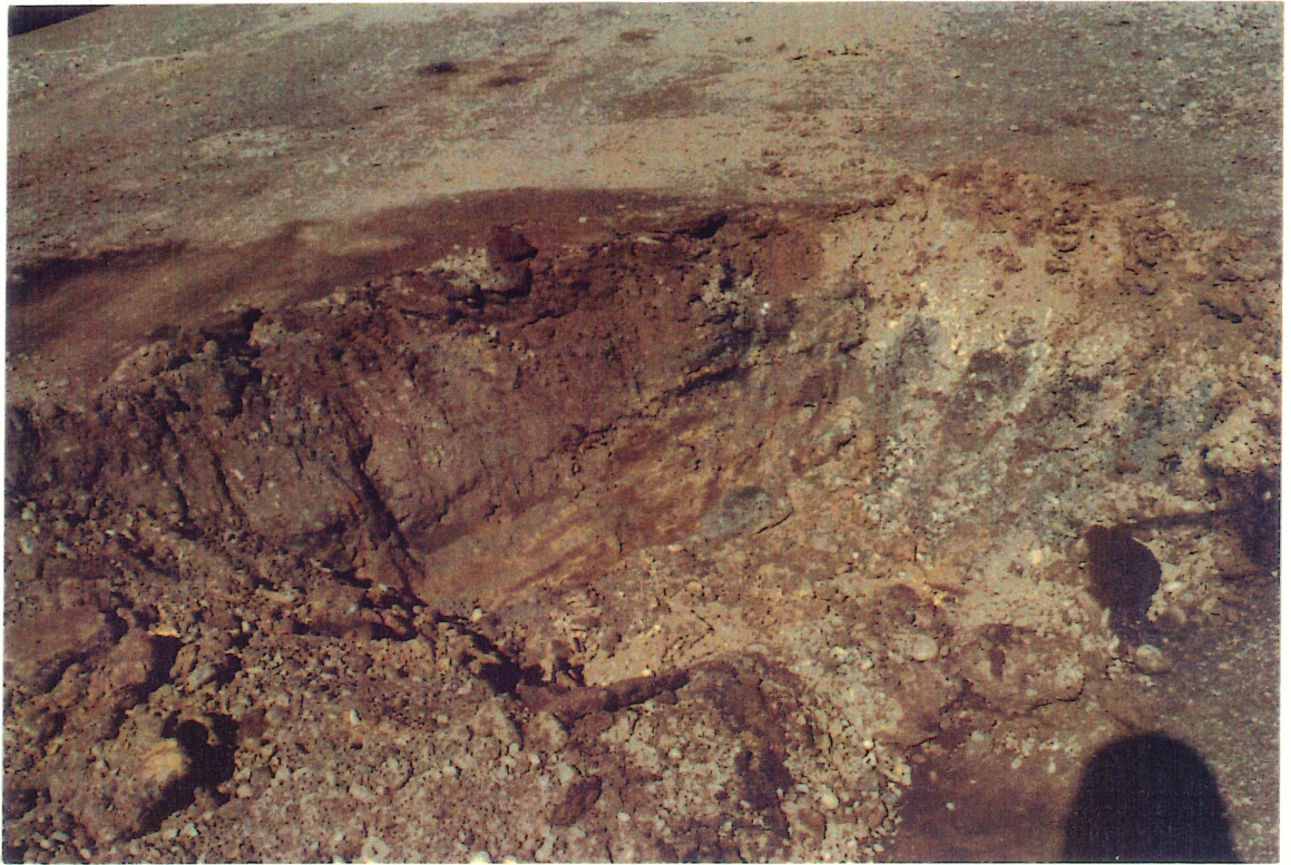
Figure 12: Villas site test pit V-TP-1. Sand and gravel fill material, stained at the surface, is underlain at 1.5 feet below grade by sandstone.
