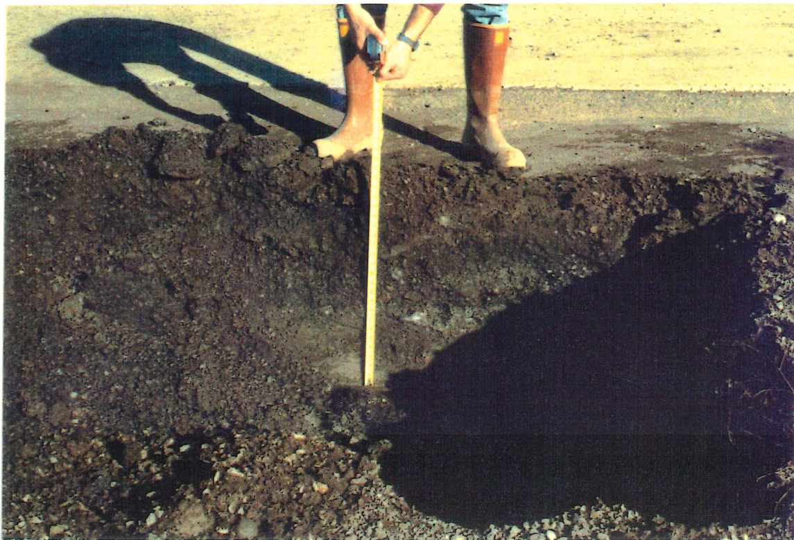
Figure 14: Visually contaminated gravelly silt layer on the Villas site.
