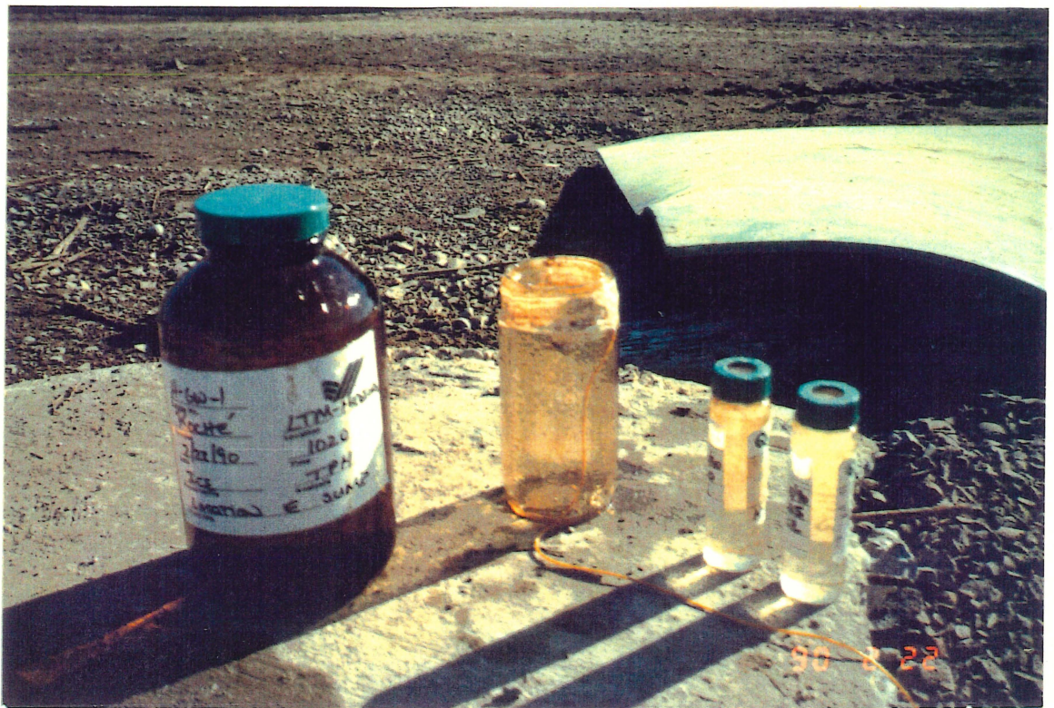
Figure 5: Bottle coated with petroleum product after being used to sample groundwater sump H-GW-1 on the Hamrick site.
