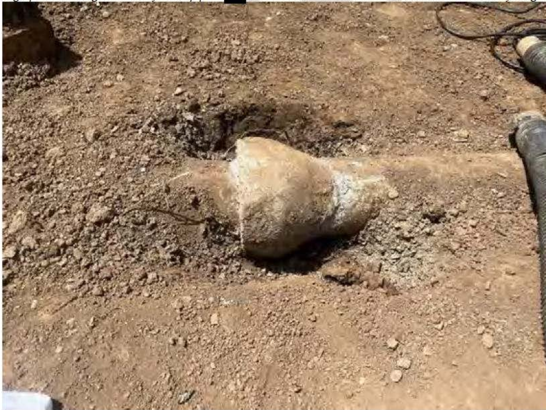
Photograph 18. Damaged section of sewer pipe at [REDACTED] Baxter connected with concrete adhesive. Photo taken facing west.
