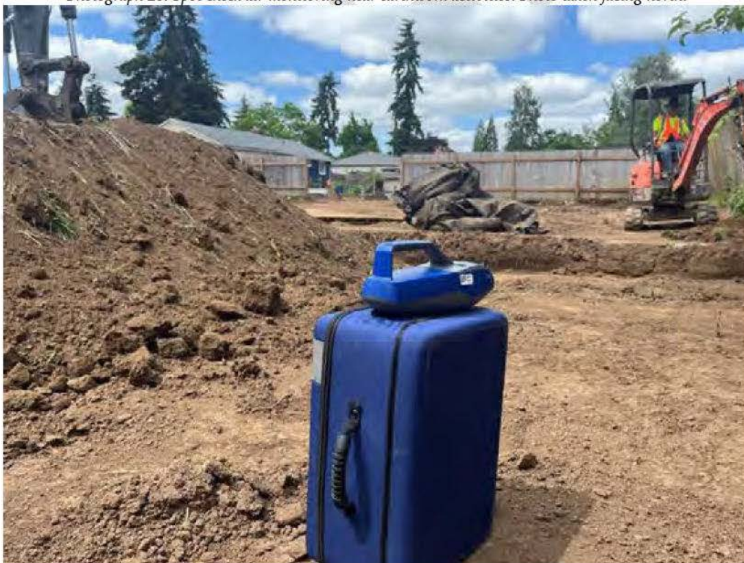
Photograph 26. Spot check air monitoring near earthwork activities. Photo taken facing north.
