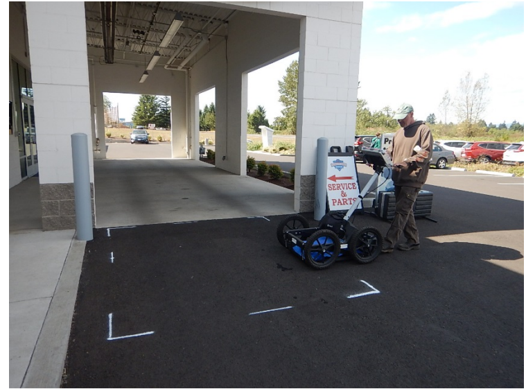
View of magnetic anomaly MA03, interpreted as a former used oil UST area.
