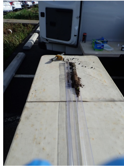
Soil cores retrieved from the drill string were inspected and field screened continuously from the surface to the total depth of each boring.
