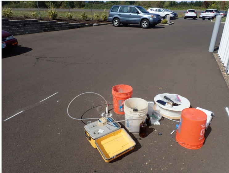
Ground water samples were collected from select borings using a peristaltic pump and dedicated tubing placed in a temporary well casing. Each well was purged prior to sampling.
