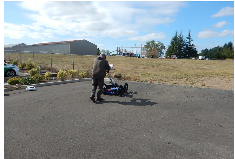
View of magnetic anomaly MA02. Disturbed soils were indicated beneath this area, interpreted to be part of the former Evaporation Pond.
