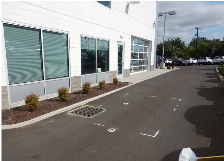
View of magnetic anomaly MA01, interpreted to be the excavation of a reported former gasoline UST.
