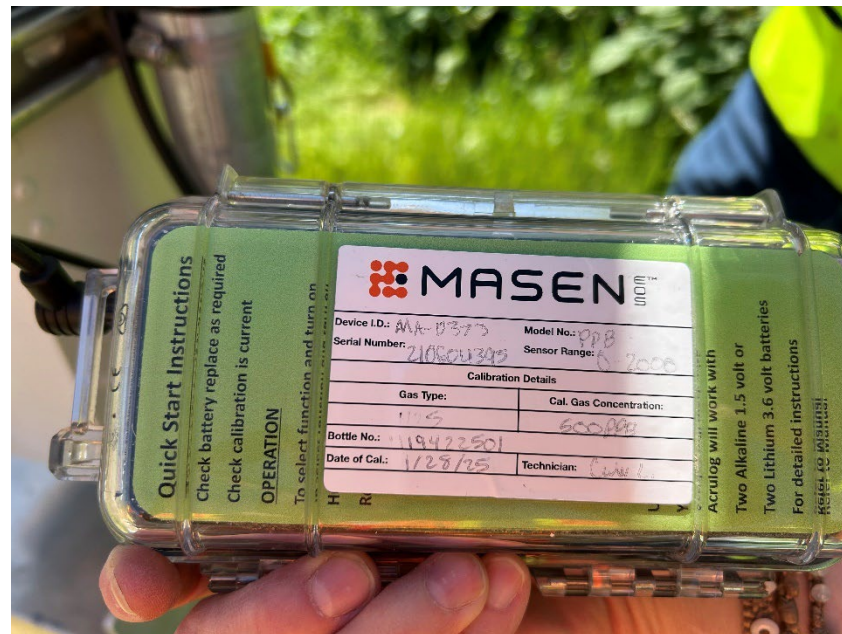
22: H2S sampling monitor. Near SW corner of ponds (SW corner of Thermal Pond C along river). Information on sampler.
