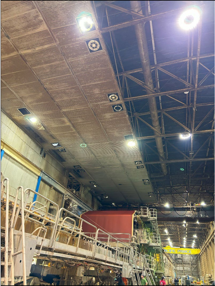
Photo 1: View of one of the paper machines. Fans in the drop ceiling, above, pull emissions through rooftop vents.
