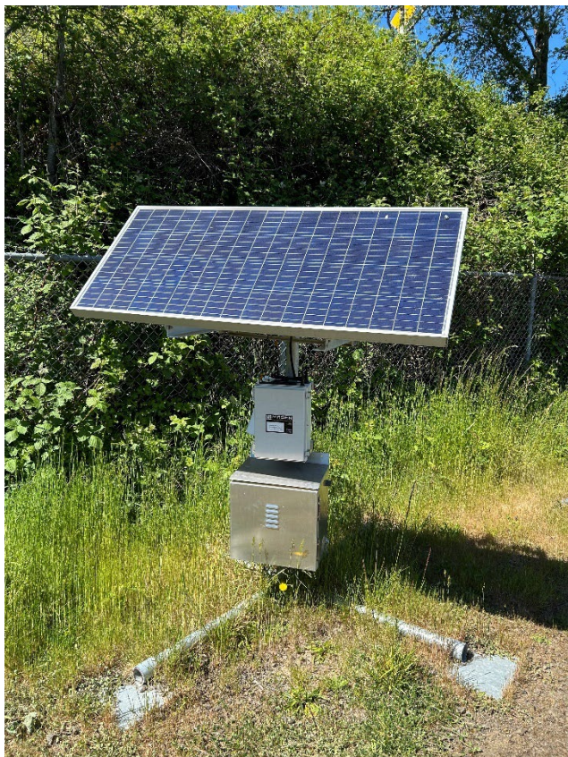
21: H2S sampling monitor. Near SW corner of ponds (SW corner of Thermal Pond C along river).
