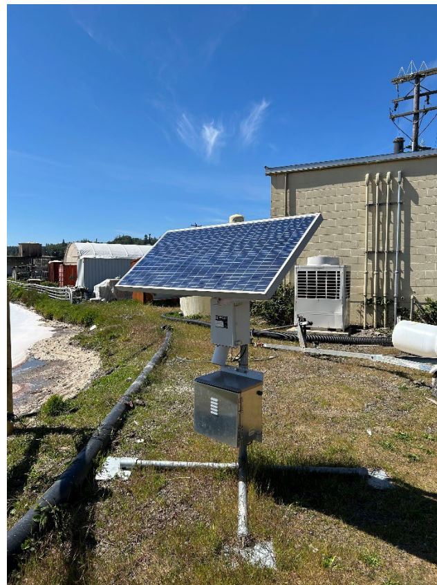
8: H2S sampling monitor. Near NW corner of Treatment Pond B.
