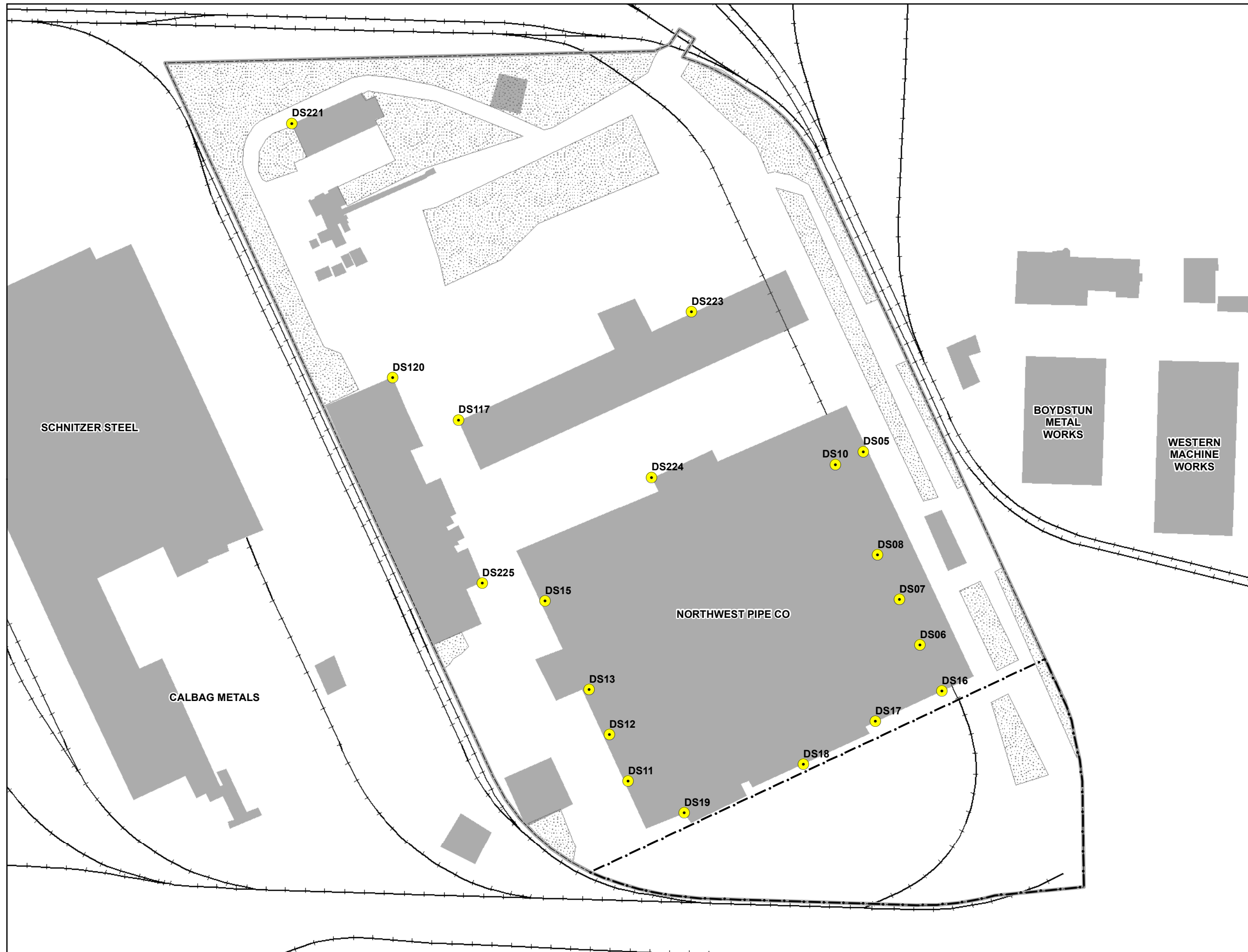
Figure 2 Downspout Roof Run-Off Sample Locations Northwest Pipe Company Portland, Oregon
