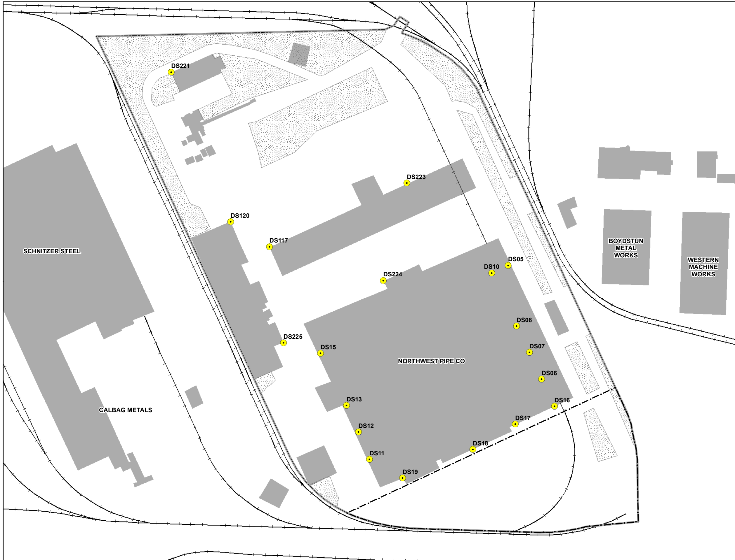
Figure 5-18 Downspout Roof Run-Off Sample Locations Northwest Pipe Company Portland, Oregon
