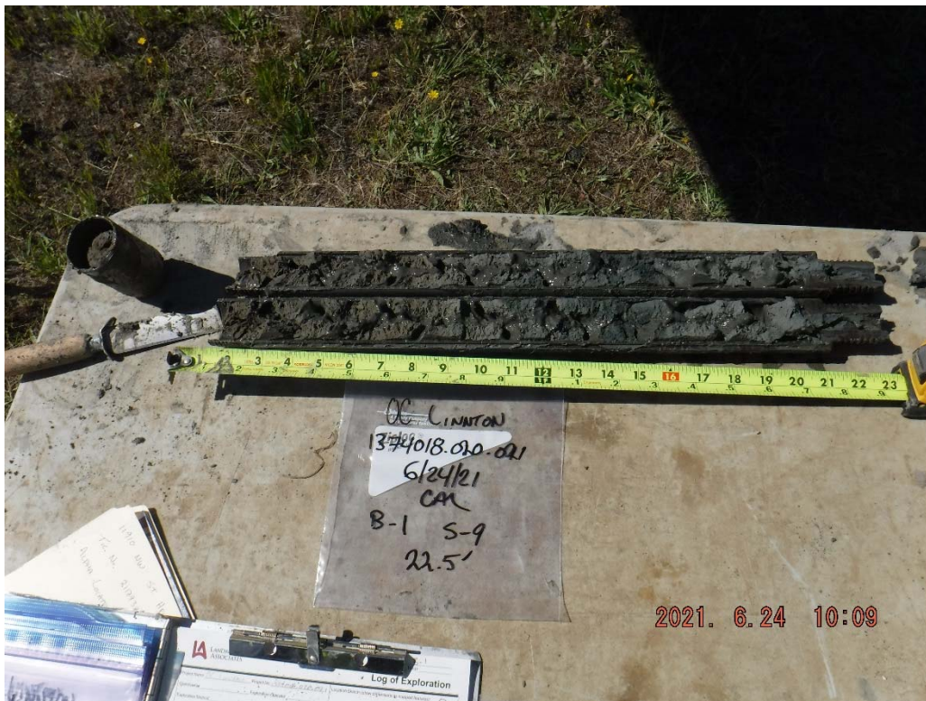
7. Boring B-1 at 22.5 feet: Gray, elastic SILT with trace organics.
