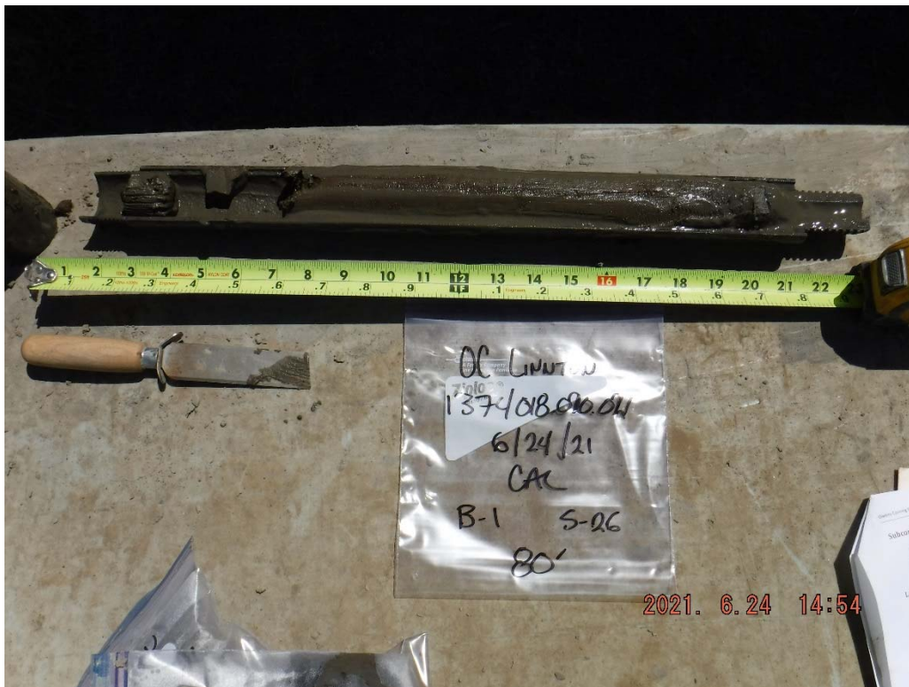
21. Boring B-1 at 80 feet: Brown, very silty, fine to medium SAND.
