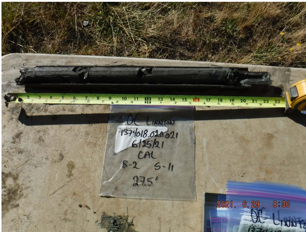
33. Boring B-2 at 27.5 feet: Dark gray SILT.
