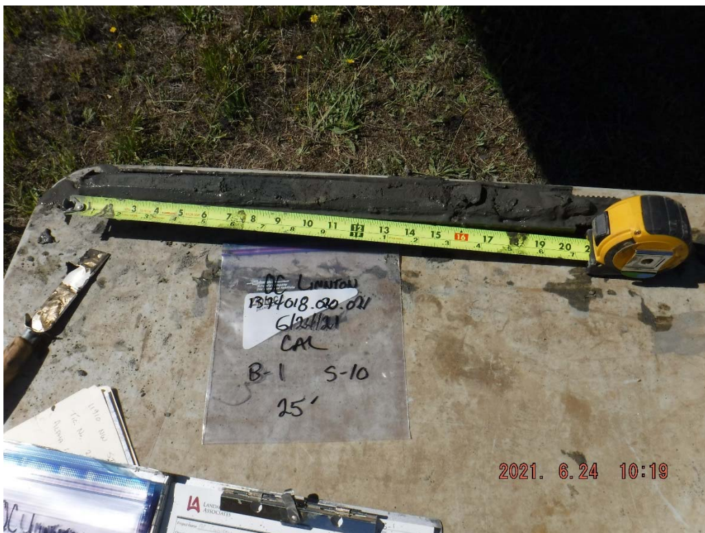
8. Boring B-1 at 25 feet: Gray, elastic SILT with trace organics.
