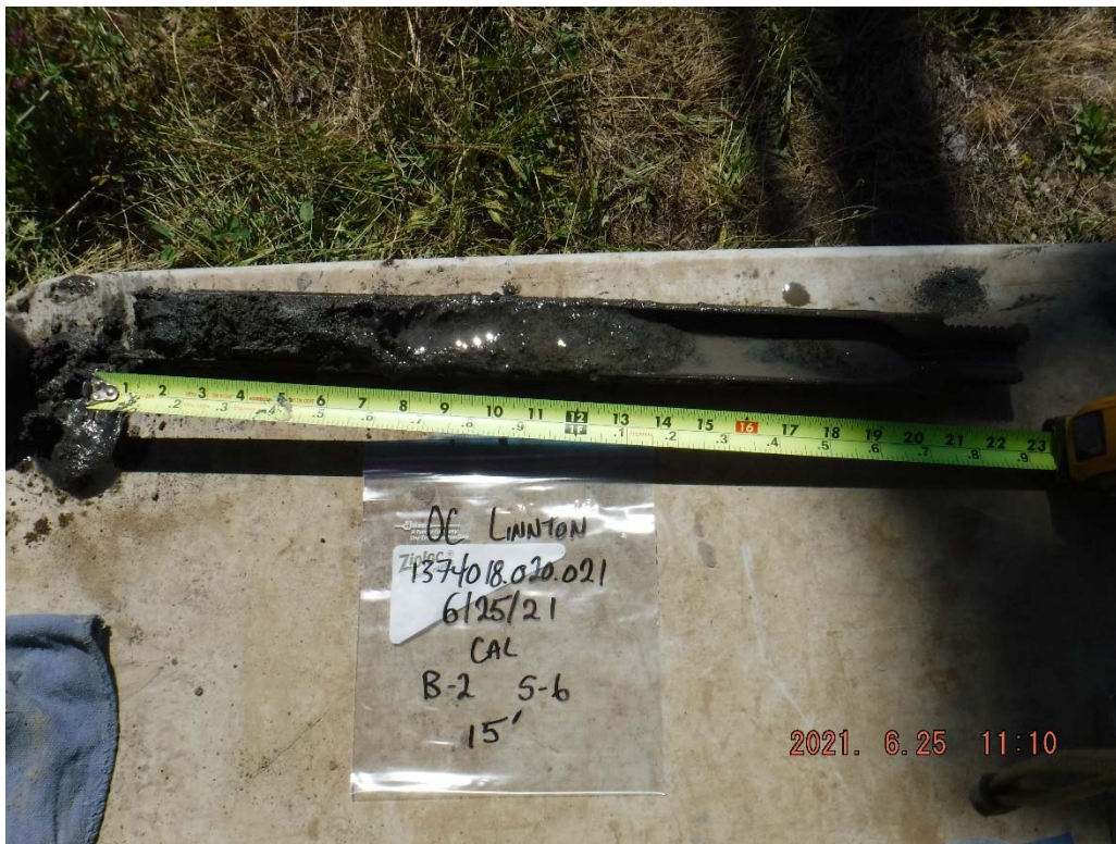
29. Boring B-2 at 15 feet: Dark gray to gray, fine to coarse SAND with gravel and silt.
