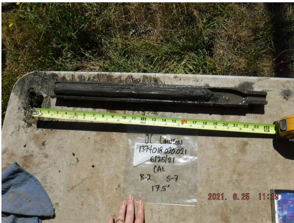
30. Boring B-2 at 17.5 feet: Gray SILT with trace organics.
