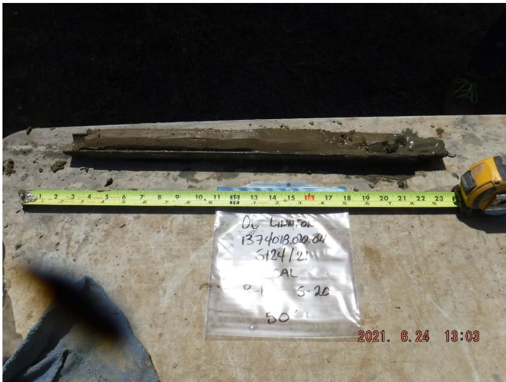
15. Boring B-1 at 50 feet: Gray-brown to brown SILT.
