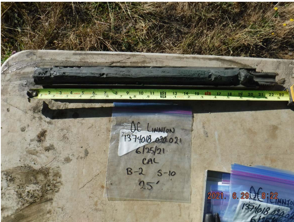
32. Boring B-2 at 25 feet: Gray, elastic SILT.
