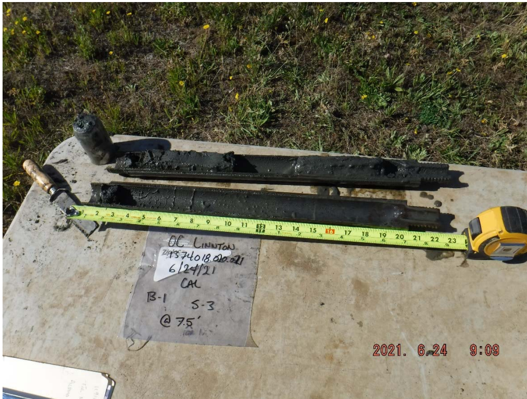
3. Boring B-1 at 7.5 feet: Gray SILT.
