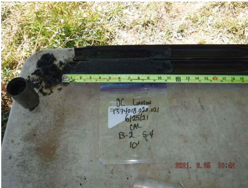
27. Boring B-2 at 10 feet: Dark gray to gray, fine to coarse SAND with gravel and silt.
