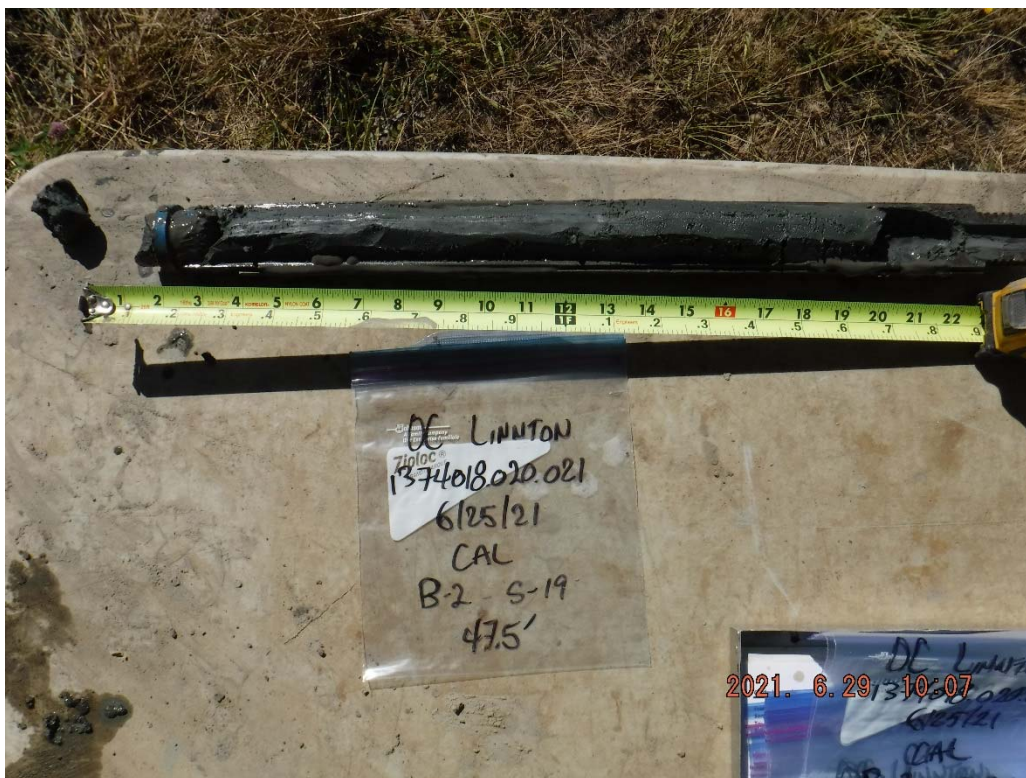
40. Boring B-2 at 47.5 feet: Light gray to blue-gray SILT.
