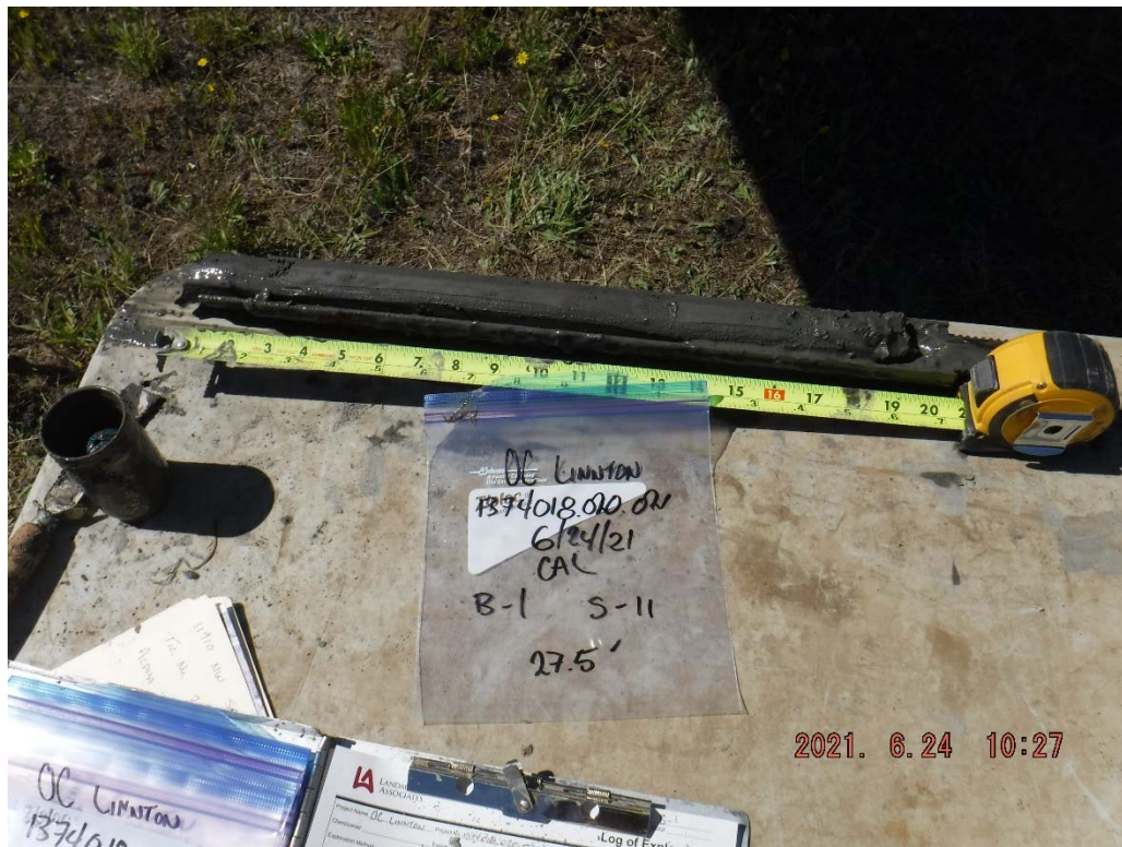
9. Boring B-1 at 27.5 feet: Dark gray SILT.
