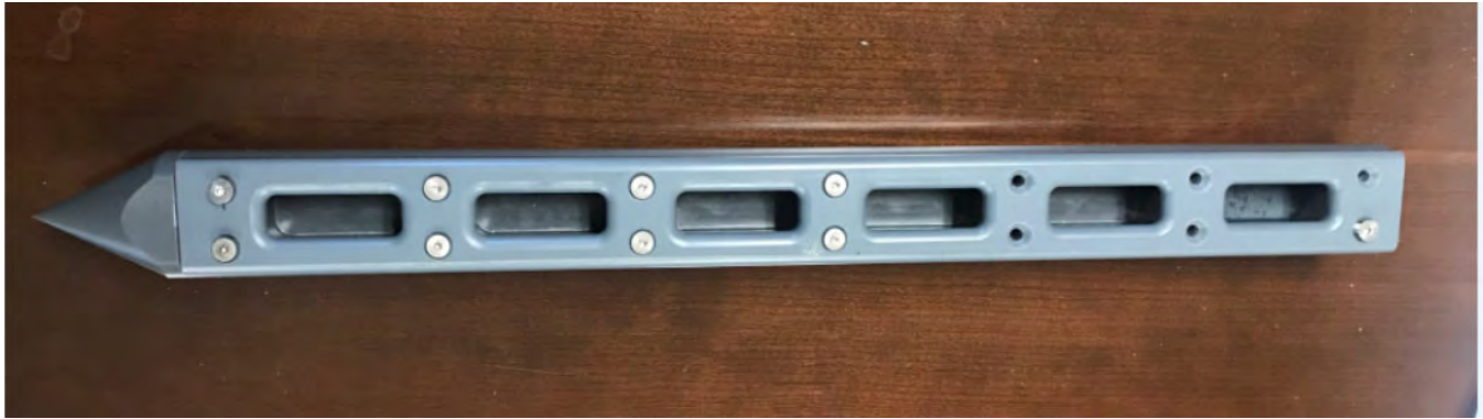
Figure 3: One passive sampling device will include sampling locations for surface water, interarmor and subarmor samples.
