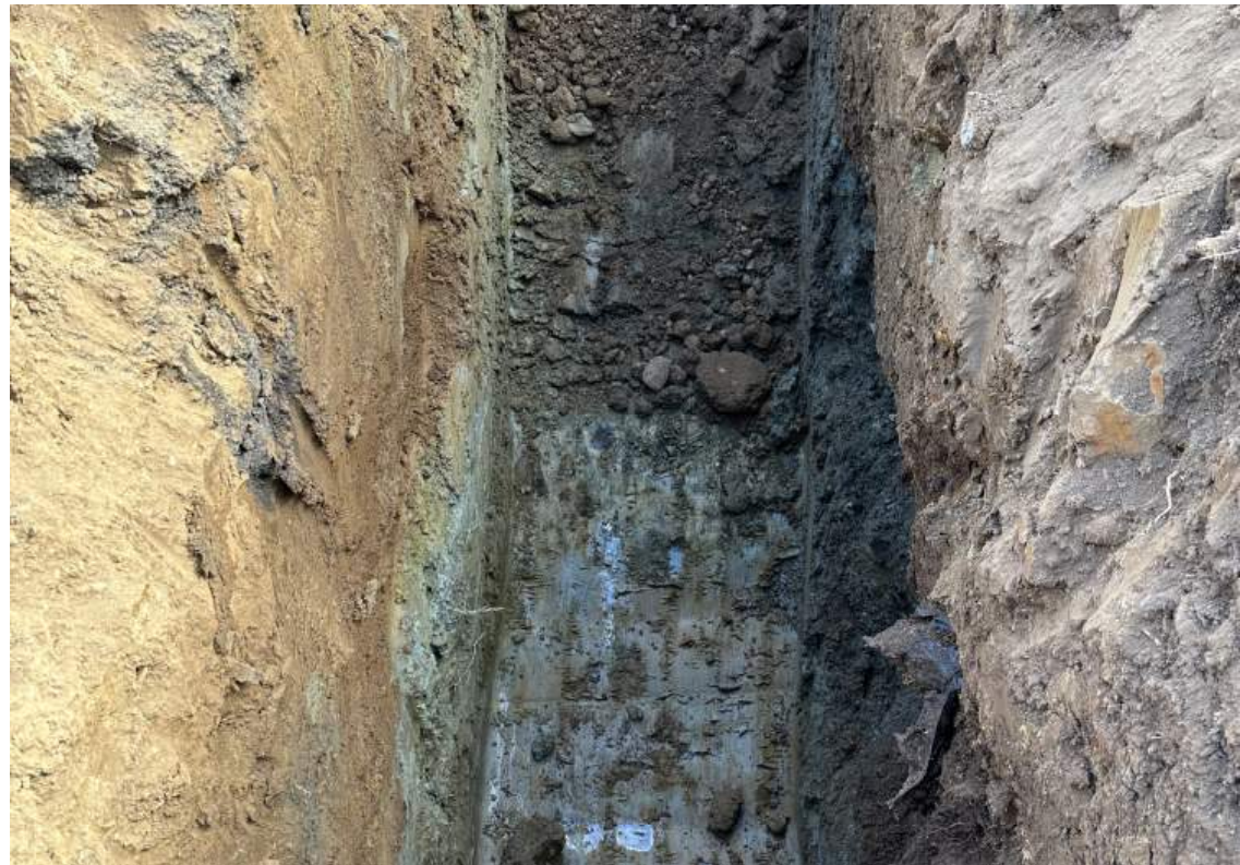
ONSITE TEST PIT "TP-1" SHOWN BELOW FORMER DRAIN PIPE DURING EXPLORATION. PHOTOGRAPH TAKEN FACING NORTH.
