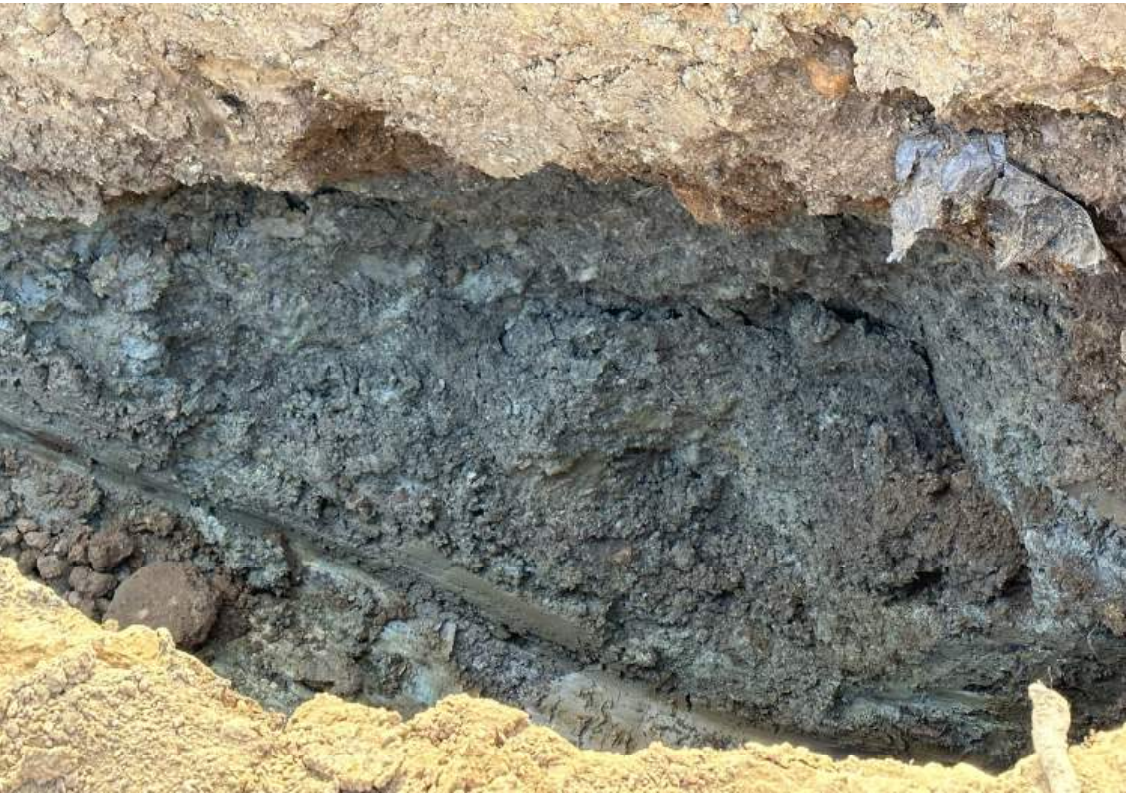
VIEW OF IMPACTED SOIL ENCOUNTERED DURING EXPLORATION OF ONSITE TEST PIT "TP-1" TAKEN FACING NORTHEAST. THIS MATERIAL WAS LATER EXCAVATED AND DISPOSED OF.
