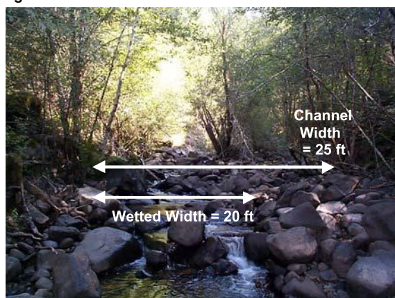
Figure 12.4 Channel width measurement
