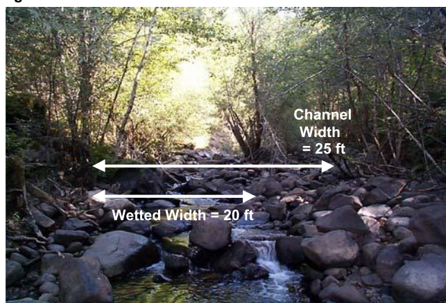
Figure 11.6 The Channel width is defined as bankfull width.
