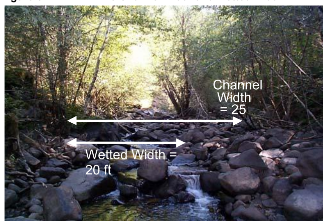
Figure 8.7. The Channel width and wetted width.
