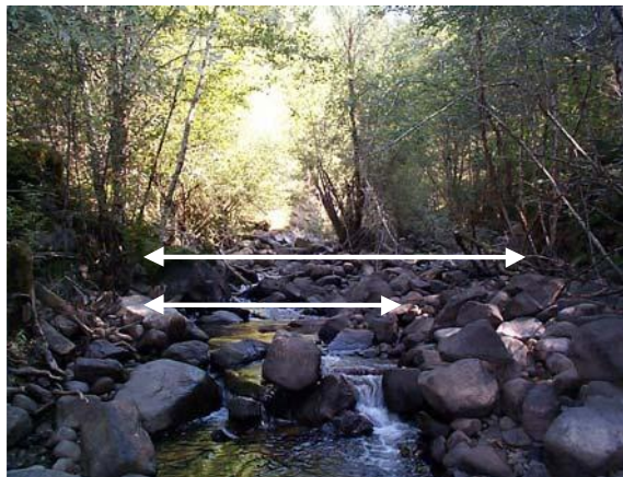
Figure 7.7 The Channel width and wetted width.
