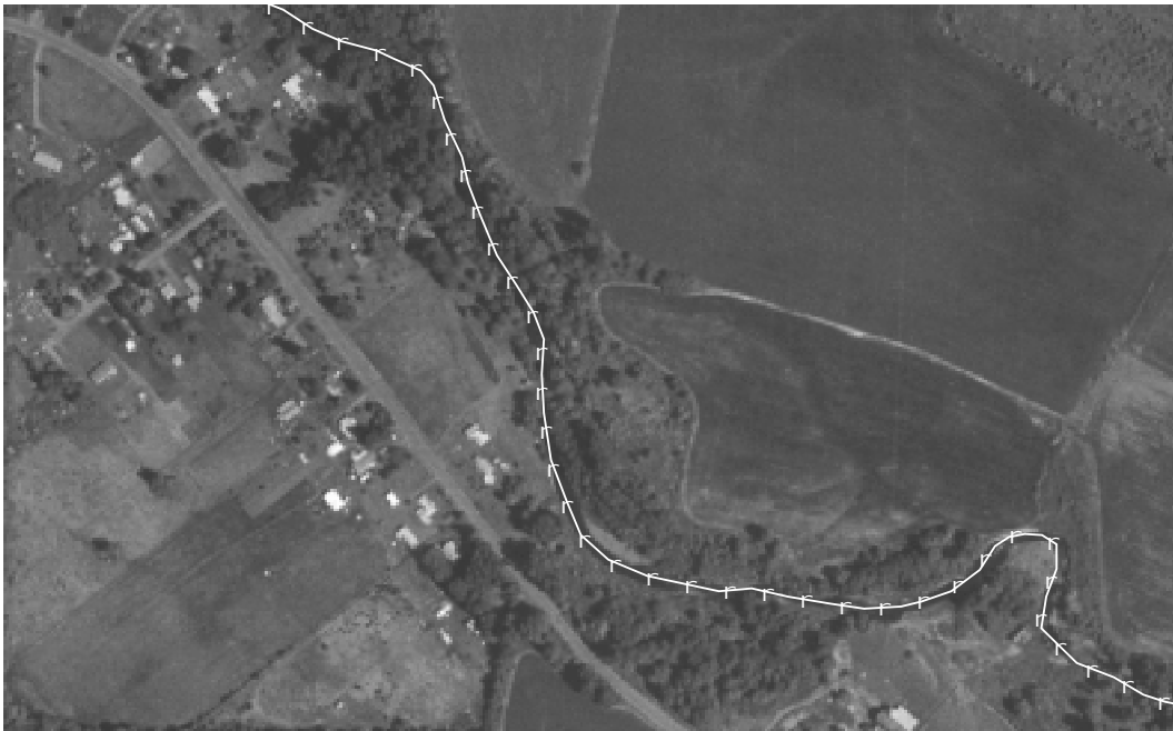
Figure A-22. Model Methodology - Stream Digitization and 100-Foot Reach Breaks on a Digital Orthophoto Quarter Quad (DOQQ) (1:3000 Scale)
