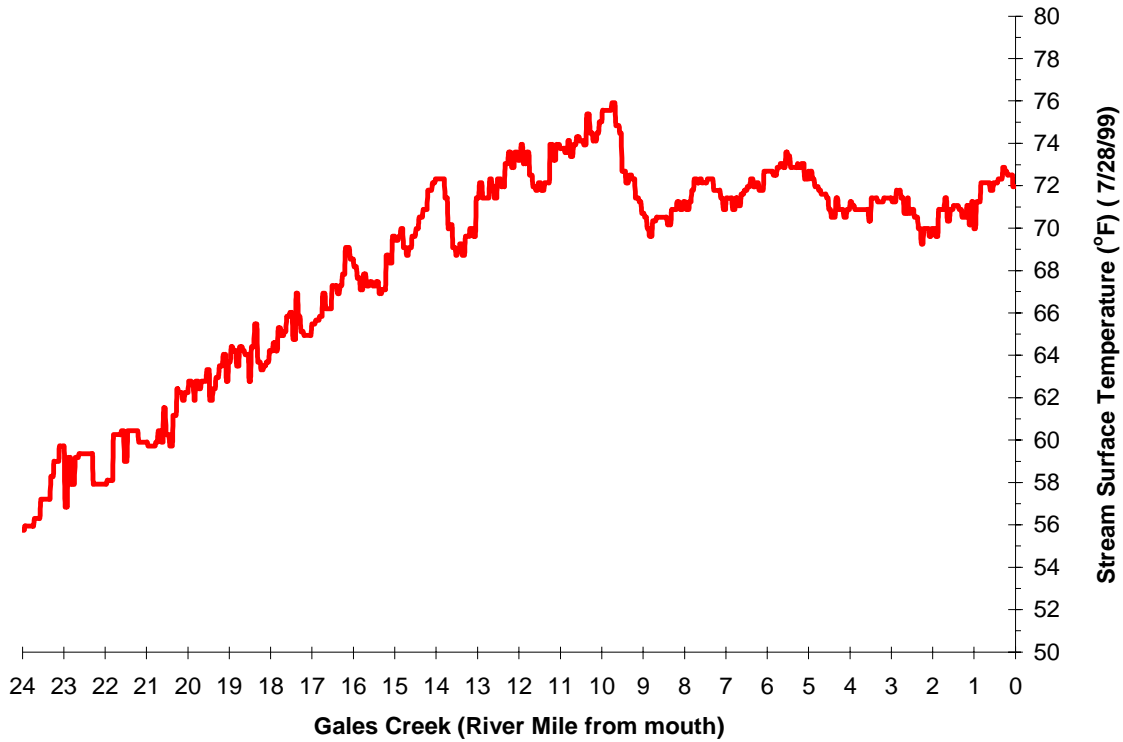
Figure A-59. Measured FLIR temperature profile for Gales Creek on July 28, 1999.
