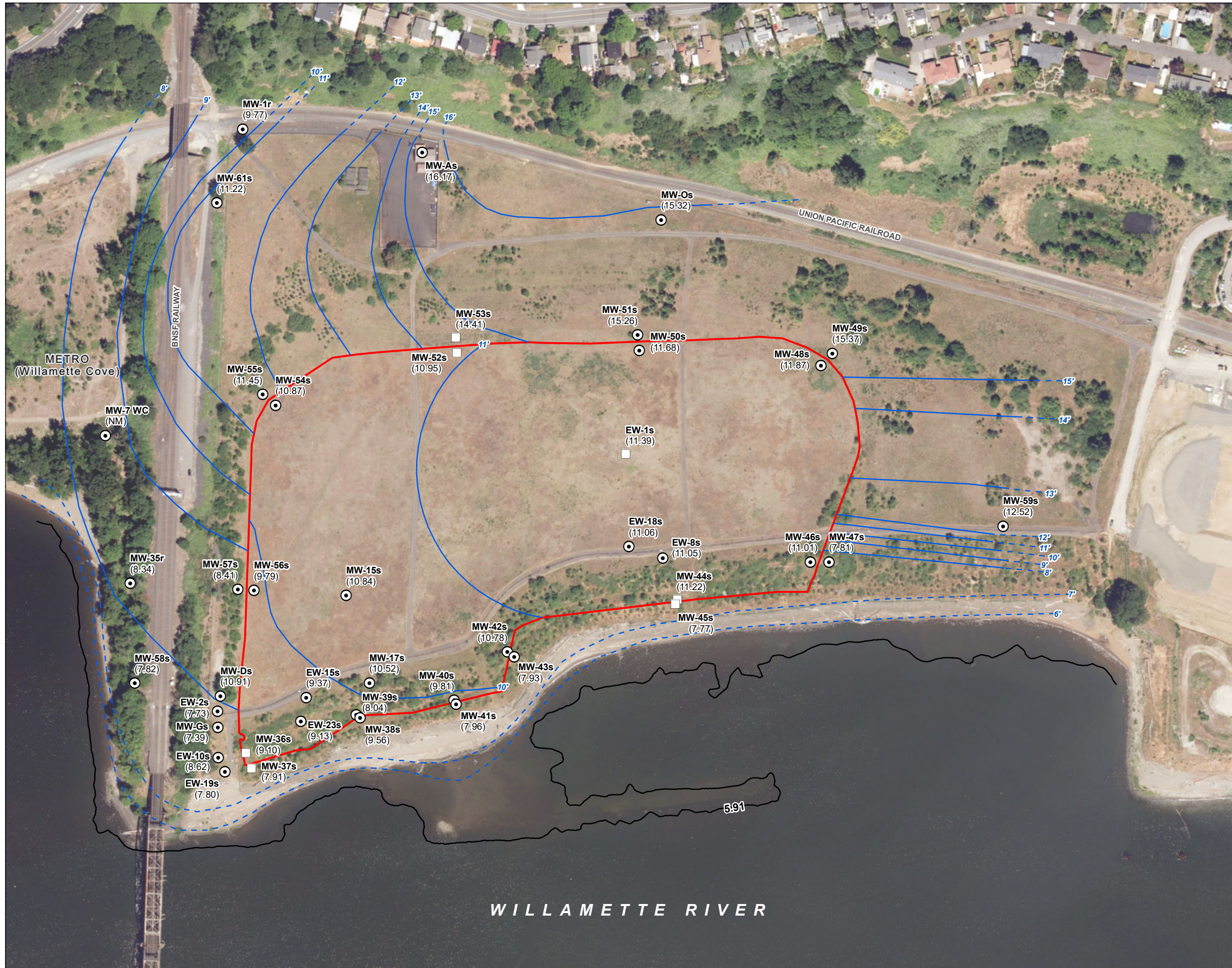
FIGURE 4-3 Groundwater Contour Map for September 2021 Monitoring Event McCormick & Baxter Superfund Site Portland, Oregon
