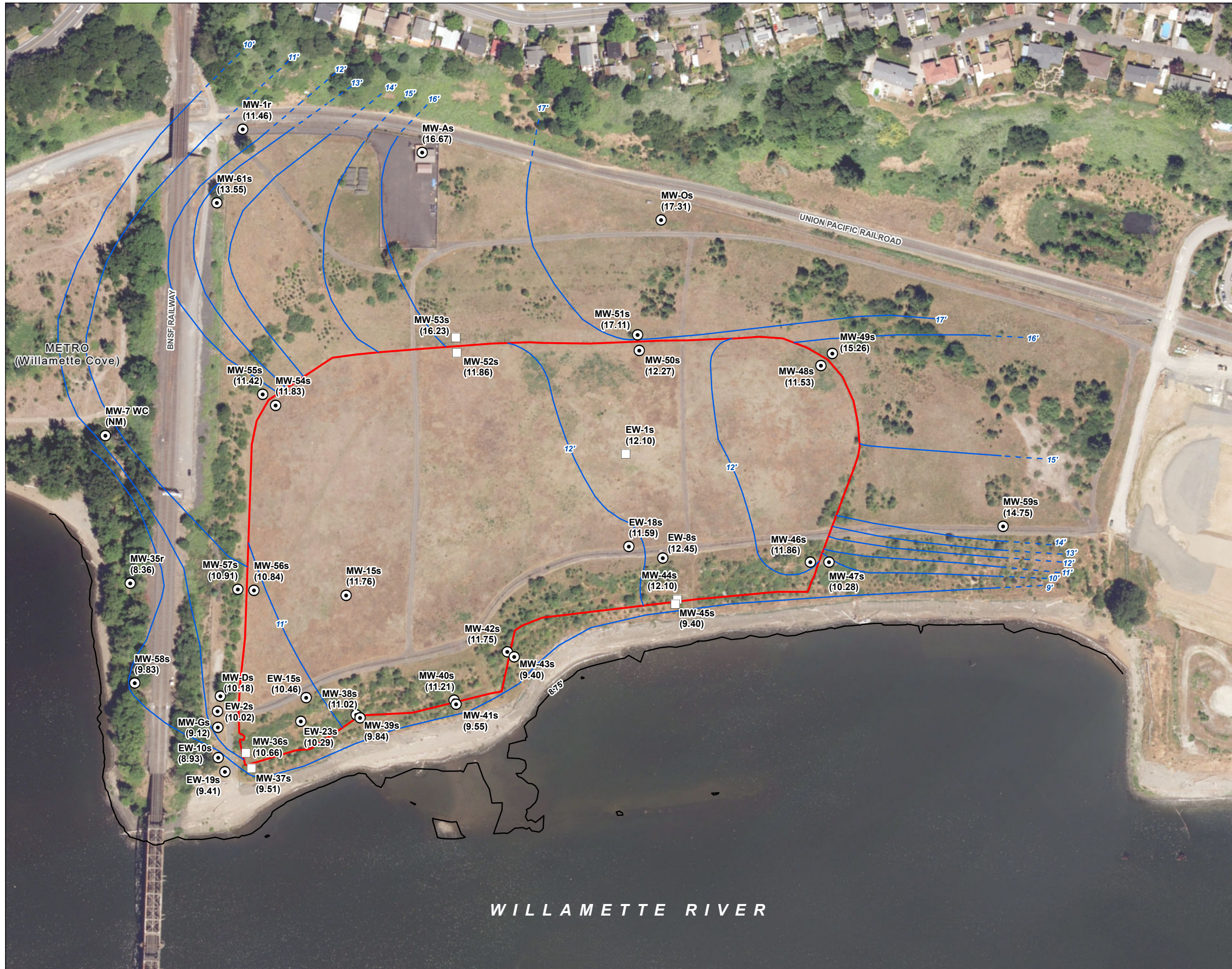
FIGURE 4-2 Groundwater Contour Map for June/July 2021 Monitoring Event McCormick & Baxter Superfund Site Portland, Oregon
