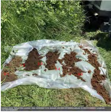
Picture taken at: 13:12 Caption: LPR-SBUST-2 hand auger cuttings Latitude: 45.42547274286829 Longitude: -123.7843769369285
