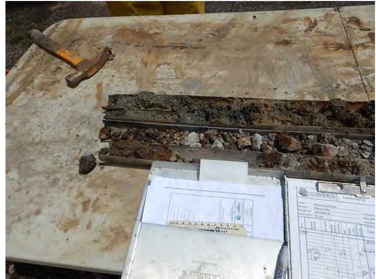
Core from EB07: wet soils in the upper core were from the soil horizon where the temporary well screen was set for sampling.
