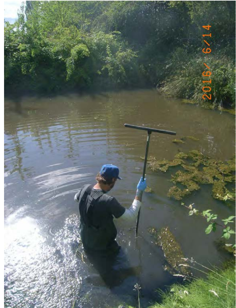
Worker using a decontaminated stainless-steel sediment push probe fitted with a long extension handle to sample pond sediment within DU03. The water was too deep to sample from the pond's center. A total of 10 sample increments were collected, composited and submitted for analytical testing.
