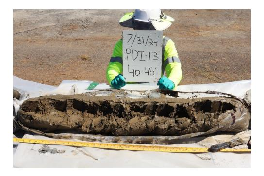
Photo 9: Phase 1 - Deep Zone - Silt with clay (PDI-13 at a depth of 40-45 feet bgs)
