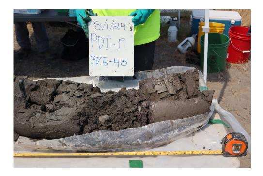
Photo 7: Phase 1 - Shallow-Intermediate Silt Zone - Interbedded sand and silt (PDI-19 at a depth of 37.5-40 feet bgs)
