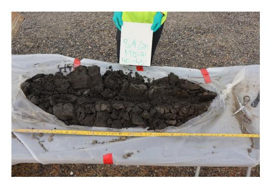
Photo 8: Phase 1 - Intermediate Zone - Fine sand with clay (PDI-21 at a depth of 40-45 feet bgs)
