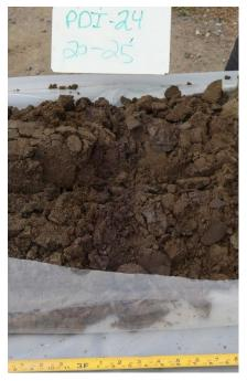
Photo 13: Phase 1 - Suspected Pesticide- and Petroleum-related Contamination collected at PDI-24 from 23.1 feet bgs within the fill material of the Vadose Zone.
