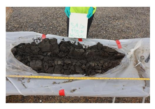
Photo 10: Phase 1 - "No Evidence of dense nonaqueous-phase liquid (DNAPL) Contamination" treatability sample collected from 41.5-42.5 feet bgs at PDI-21 within the fine sand with clay unit of the Intermediate Zone.
