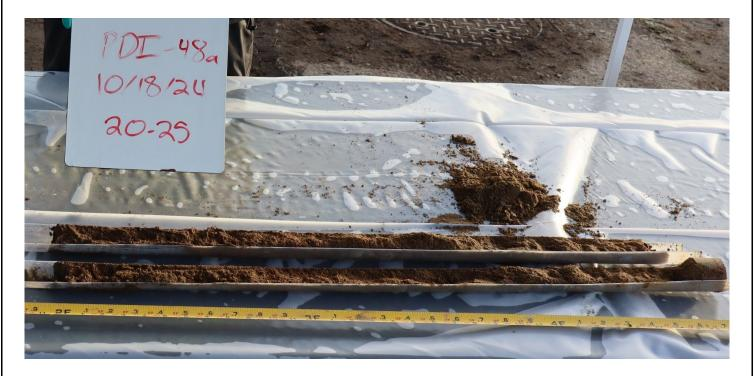
Photo 17: Phase 2 - Vadose Zone - Fine-to-medium sand with silt and clay (PDI-48a at a depth of 20-25 feet bgs)
