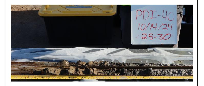
Photo 19: Phase 2 - Shallow Zone - Fill (PDI-40 at a depth of 26.5-28.3 feet bgs)
