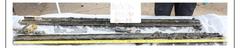
Photo 21: Phase 2 - Shallow Zone - Sandy silt (PDI-51 at a depth of 20-24.4 feet bgs)
