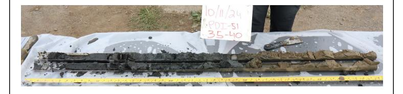
Photo 24: Phase 2 - Deep Zone - Silt with clay (PDI-51 at a depth of 35.9-40 feet bgs)
