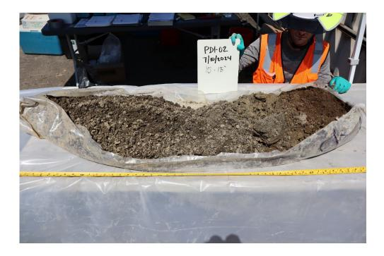
Photo 3: Phase 1 - Vadose Zone - Sandy Silt (PDI-02 at a depth of 13.8-14.3 feet bgs)
