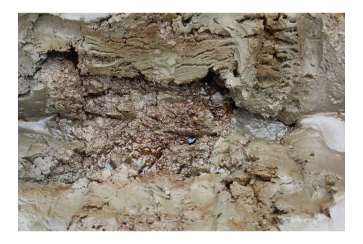
Photo 12: Phase 1 - "Contaminated" treatability sample collected from 11-12 feet bgs at PDI-13 within the sandy silt unit of the Shallow Zone.
