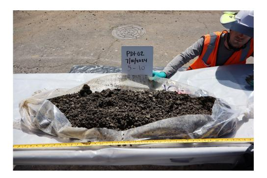
Photo 1: Phase 1 - Vadose Zone - Fill (PDI-02 at a depth of 5-10 feet below ground surface (bgs))
