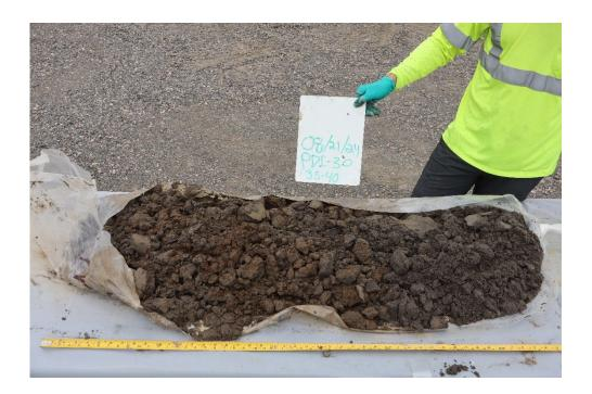
Photo 5: Phase 1 - Shallow Zone - Fine-to-medium sand with silt and clay (PDI-30 at a depth of 35-40 feet bgs)
