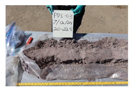
Photo 2: Phase 1 - Vadose Zone - Fine-to-medium sand with silt and clay (PDI- 03 at a depth of 20-22.5 feet bgs)
