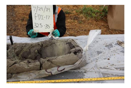
Photo 11: Phase 1 - "Some DNAPL Contamination" treatability sample collected from 33.2-34.5 feet bgs at PDI-17 within the interbedded sand and silt unit of the Shallow-Intermediate Silt Zone
