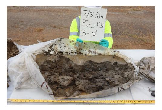
Photo 6: Phase 1 - Shallow Zone - Sandy silt (PDI-13 at a depth of 5-10 feet bgs)
