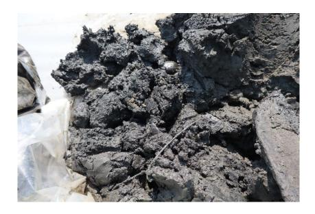
Photo 14: Phase 1 - Suspected Petroleum-based nonaqueous-phase liquid (NAPL) collected at PDI-21 from 20.2 feet bgs within the fill material of the Vadose Zone.
