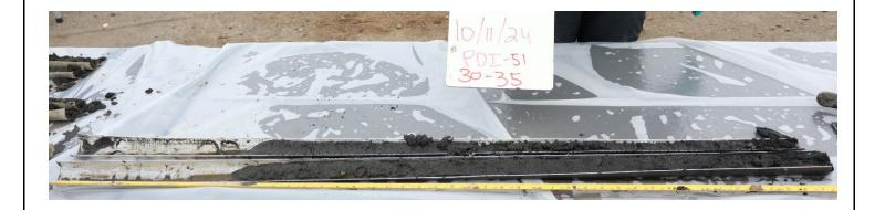
Photo 23: Phase 2 - Intermediate Zone - Fine sand with clay (PDI-51 at a depth of 30-35 feet bgs)
