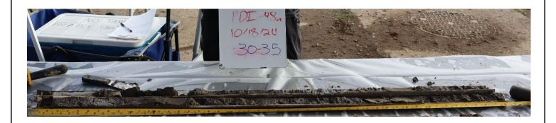
Photo 20: Phase 2 - Shallow Zone - Fine-to-medium sand with silt and clay (PDI-48a at a depth of 30-35 feet bgs)
