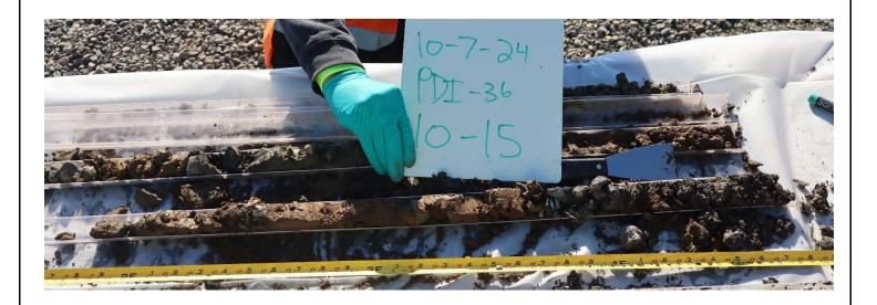
Photo 16: Phase 2 - Vadose Zone - Fill (PDI-36 at a depth of 10-15 feet bgs)
