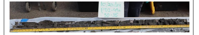
Photo 22: Phase 2 - Shallow-Intermediate Silt Zone - Interbedded sand and silt (PDI-49a at a depth of 30.5-35 feet bgs)
