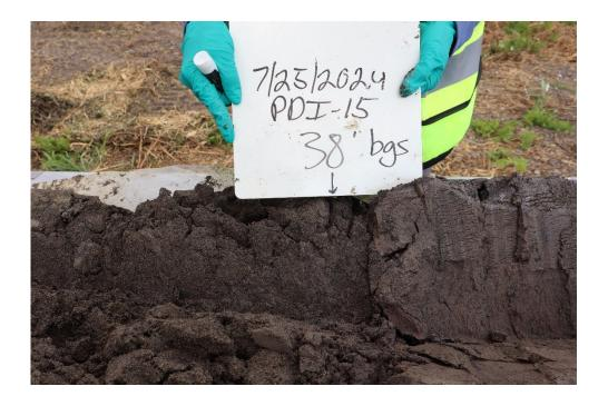
Photo 15: Phase 1 - PDI-15 Unknown Substance at 38 feet bgs on top of the interbedded sand and silt unit of the Shallow-Intermediate Silt Zone.
