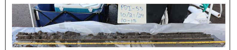
Photo 18: Phase 2 - Vadose Zone - Sandy Silt (PDI-55 at a depth of 10-15 feet bgs)
