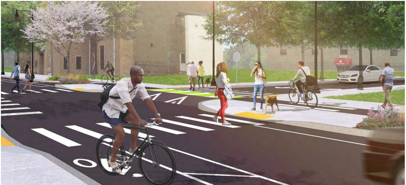
Figure 32. Example Raised Crosswalk
