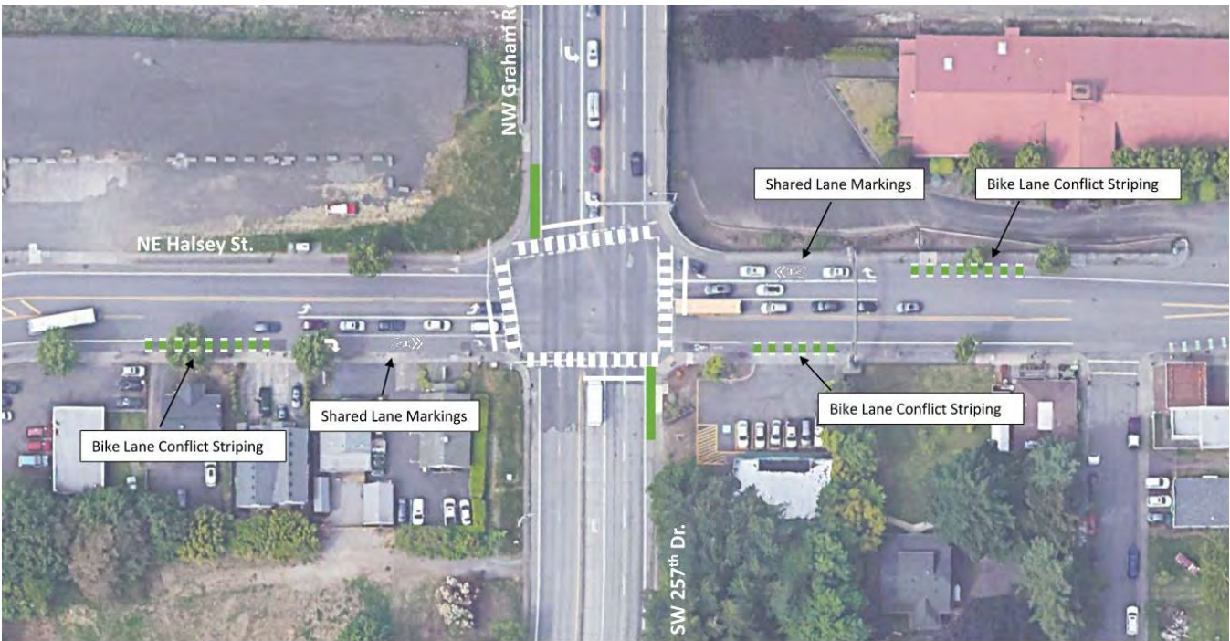
Figure 7. Near-term Intersection Treatments – SW 257 th Drive
