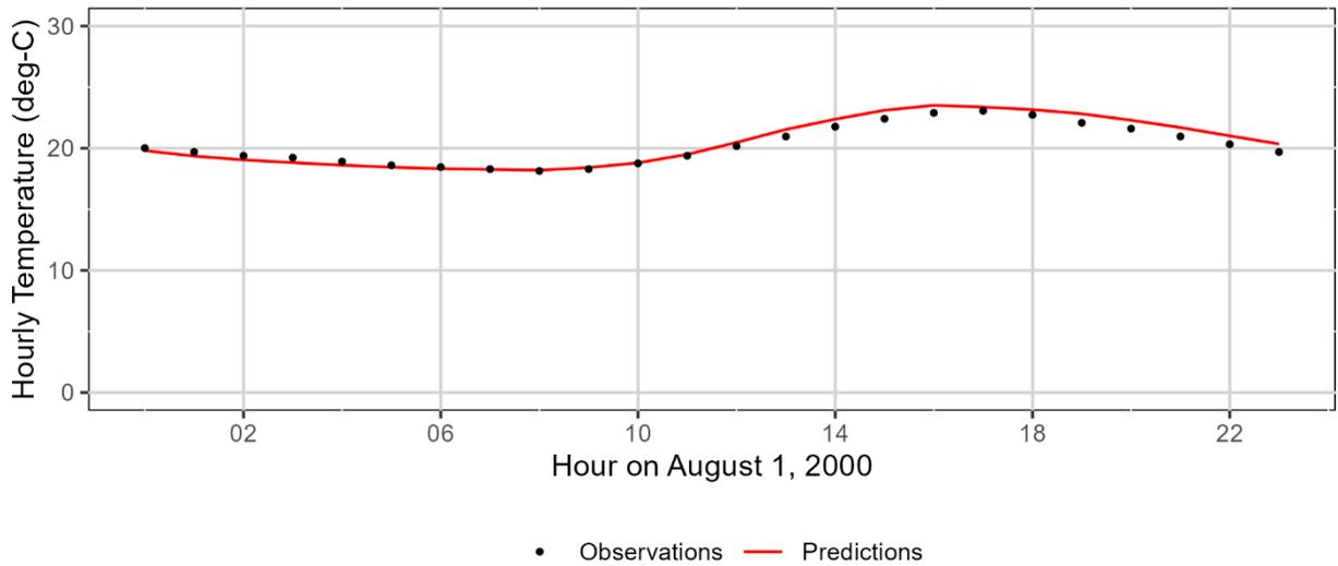
**Figure 3-108: Little North Santiam River measured and model-predicted hourly temperatures at monitoring station BLMEH.**
