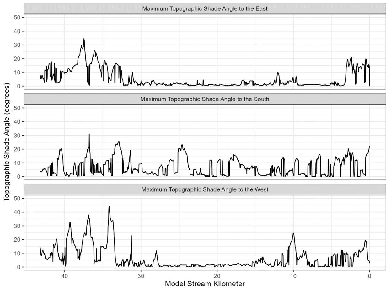
**Figure 3-206: Topographic shade angle inputs to the upper McKenzie River model.**
