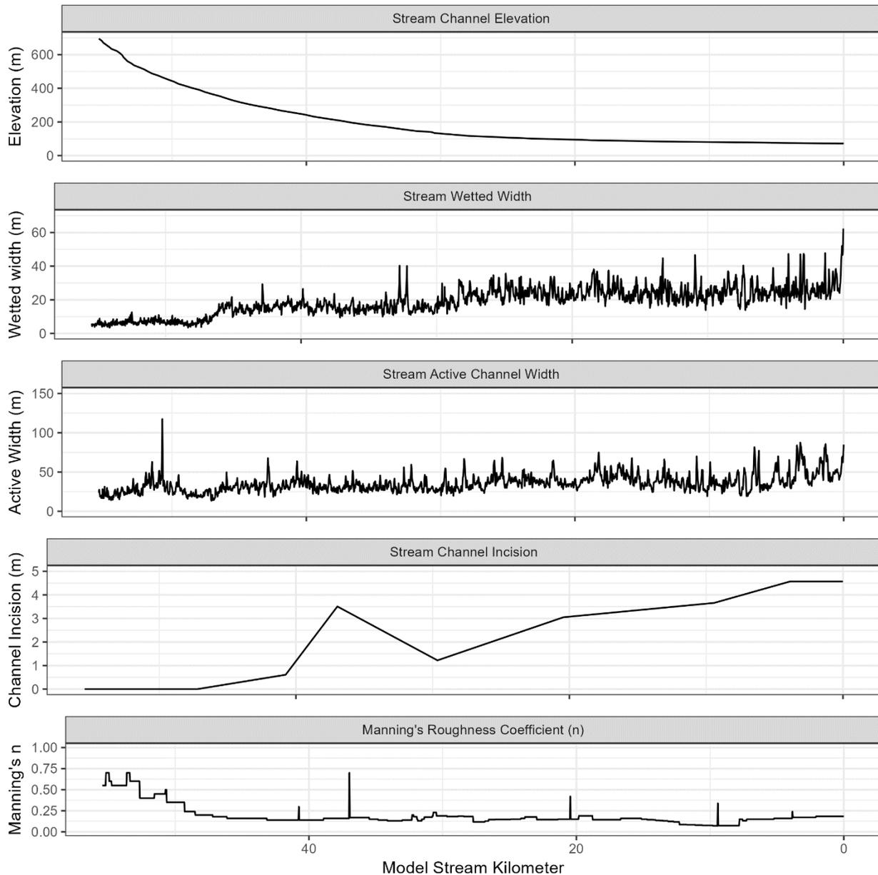
Figure 3-143: Channel setup in the Crabtree Creek model.
