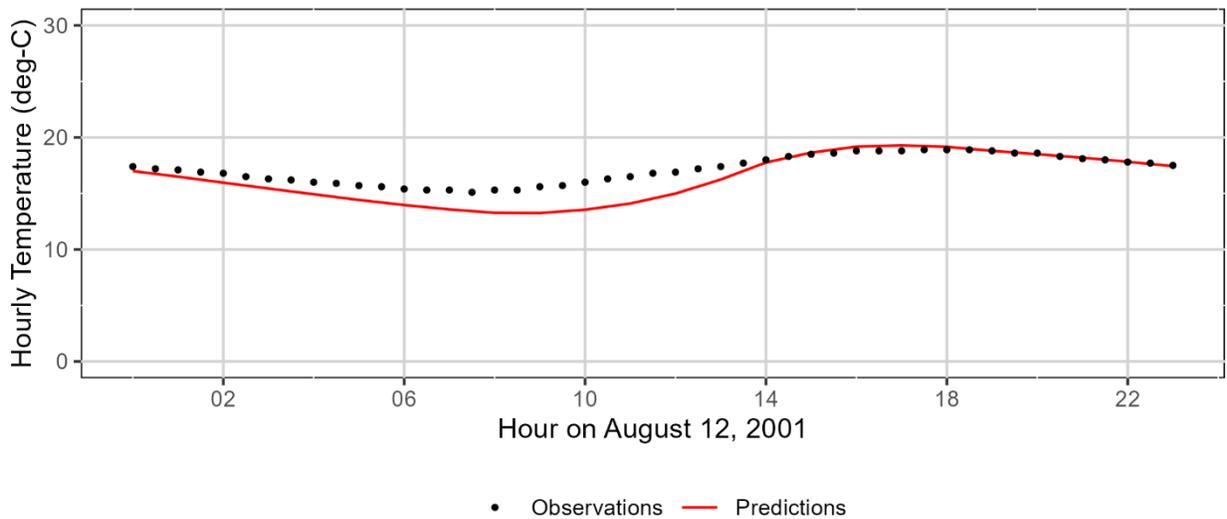
Figure 3-174: Luckiamute River measured and model-predicted hourly temperatures at monitoring station 25490-ORDEQ.
