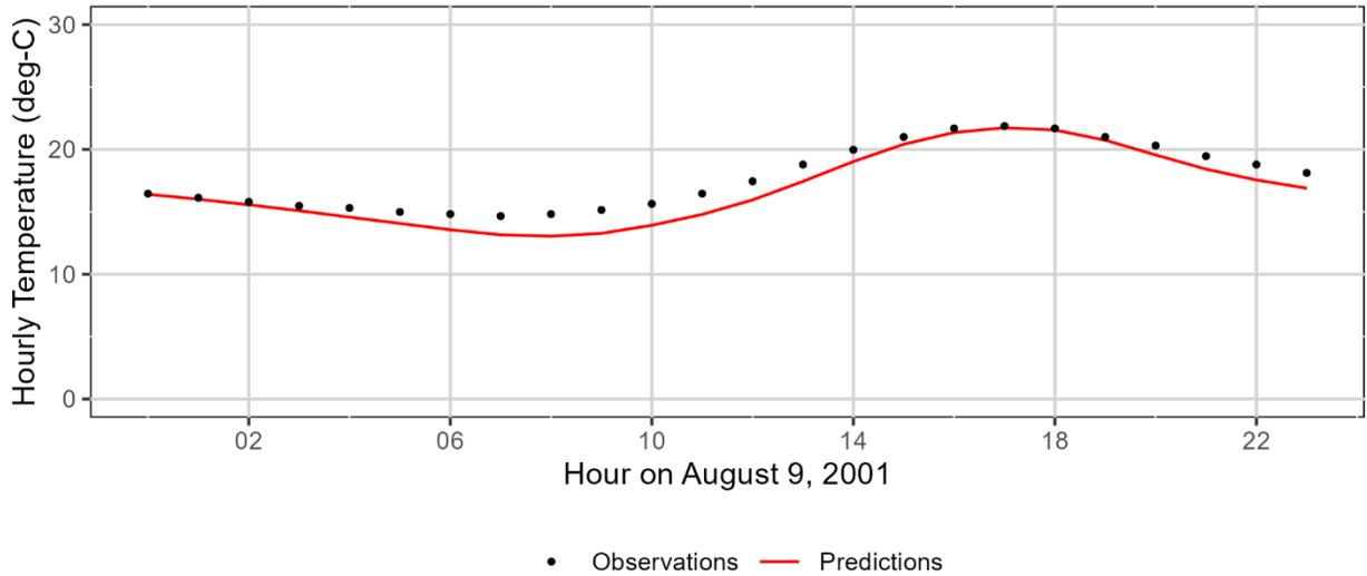
Figure 3-193: Mohawk River measured and model-predicted hourly temperatures at monitoring station 22651-ORDEQ.
