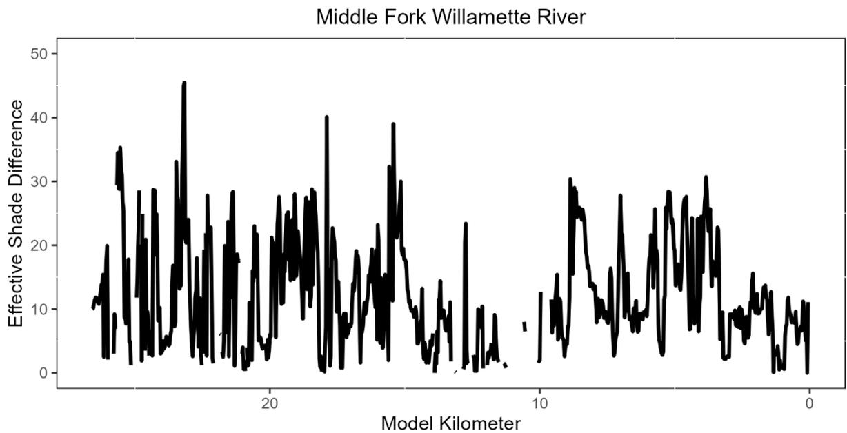
**Figure 4-97: Percentage point difference between effective shade from the Current Condition and Restored Vegetation scenarios on 7/2/2002 for the Middle Fork Willamette River. Missing values indicate that the shade difference is negative due to instances of higher effective shade in the Current Condition scenario versus the Restored Vegetation scenario.**
