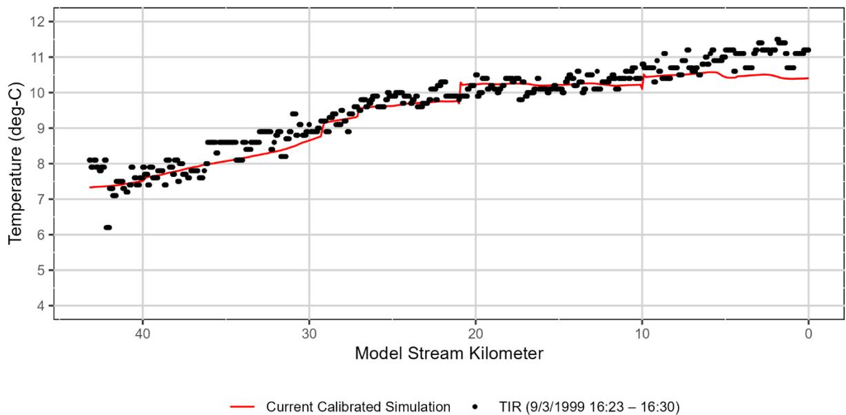
Figure 3-211: Upper McKenzie River TIR and simulated current stream temperatures.
