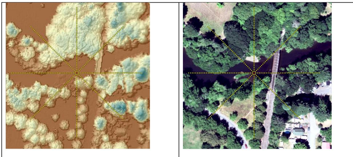
**Figure 3-248: Example of the star pattern canopy height sampling at the MAR1 sample site. LiDAR derived height on the left and the same location as depicted in 2018 aerial imagery on the right. The stream node is depicted in red at the center.**
