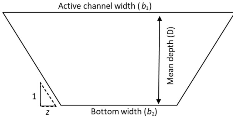
**Figure 2-11: Conceptual diagram of trapezoidal channel and terms used in Equation 2-1.**
