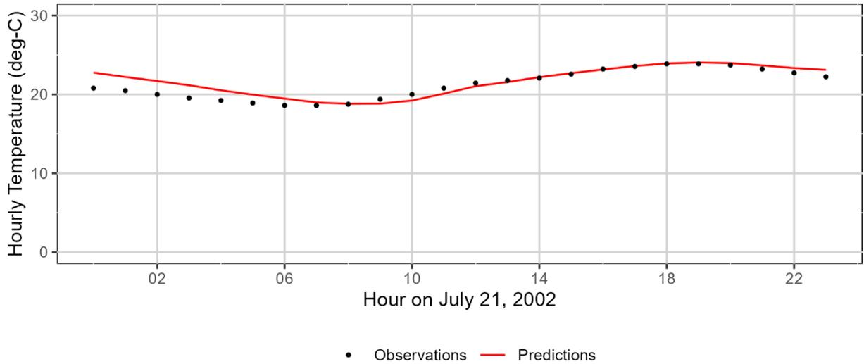
Figure 3-239: Mosby Creek measured and model-predicted hourly temperatures at monitoring station 30368-ORDEQ.
