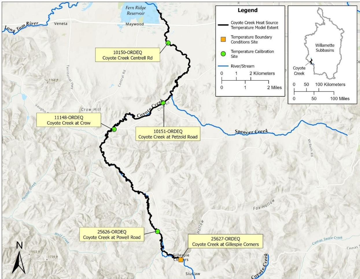
**Figure 3-215: Temperature monitoring locations used for the Coyote Creek model setup and calibration.**
