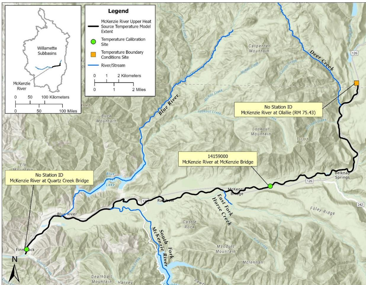
**Figure 3-200: Temperature monitoring locations used for the upper McKenzie River model setup and calibration.**
