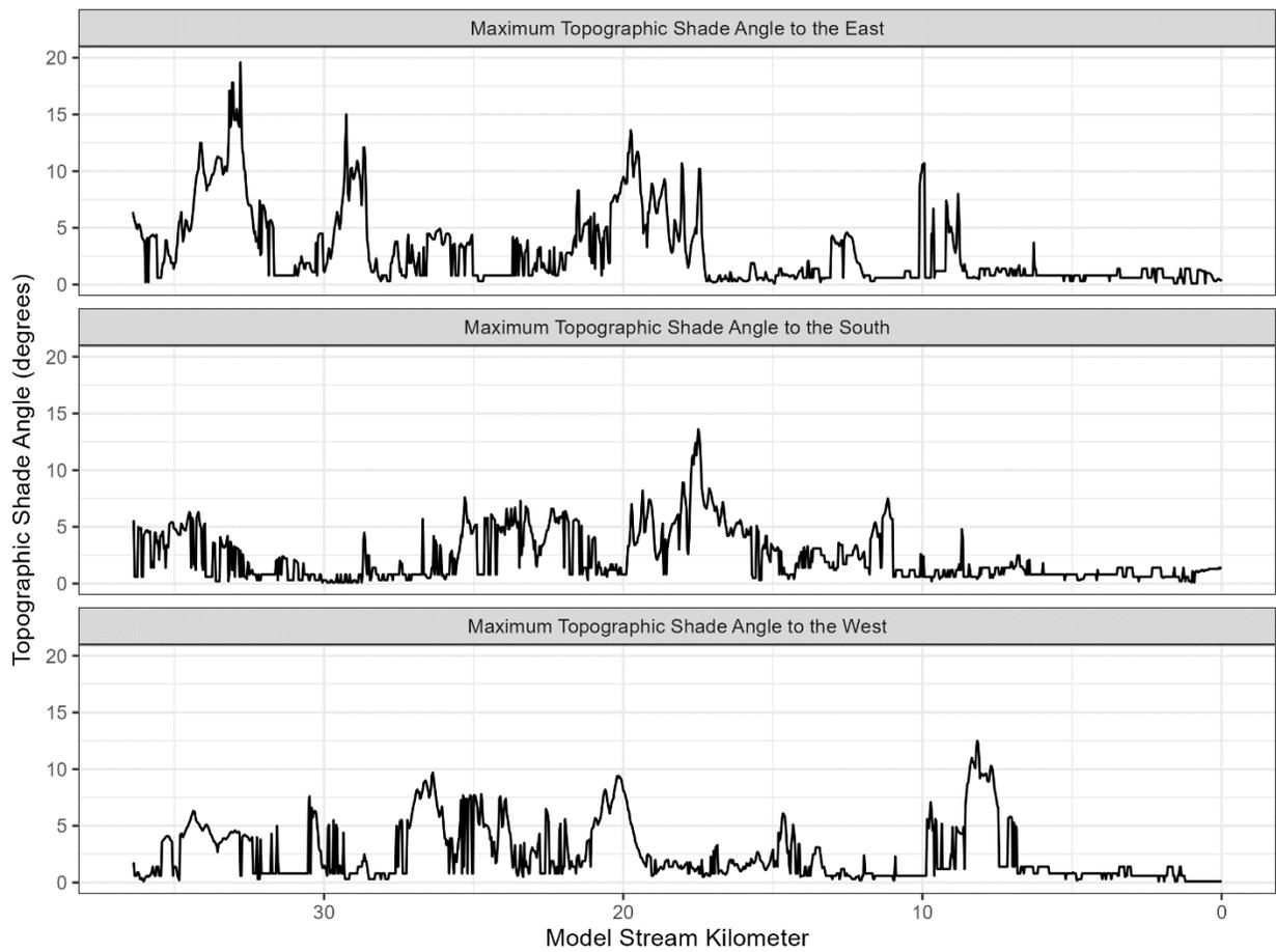
**Figure 3-220: Topographic shade angle inputs to the Coyote Creek model.**
