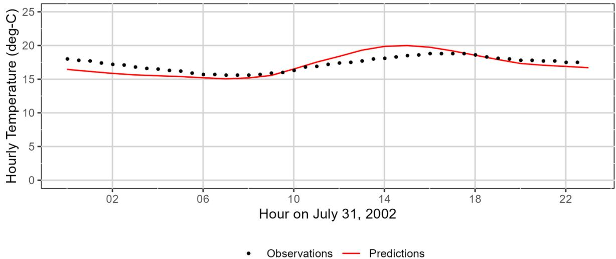
**Figure 3-15: Johnson Creek measured and model-predicted hourly temperatures at monitoring station 10856-ORDEQ.**
