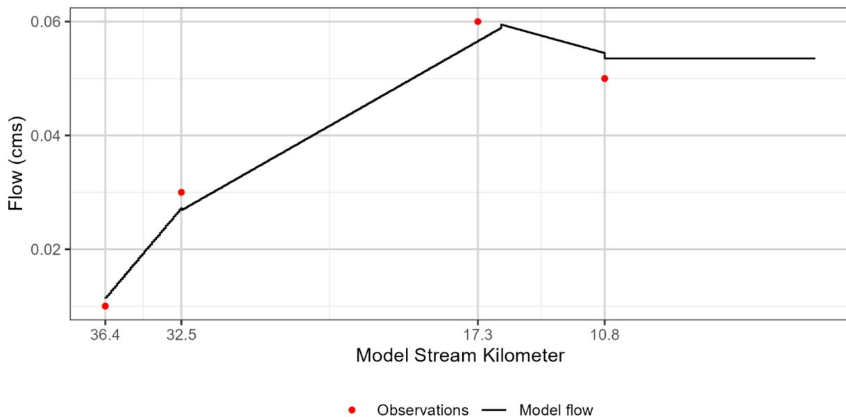
**Figure 3-227: Coyote Creek field observed and model flow rates.**
