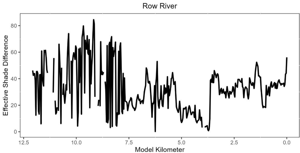
**Figure 4-101: Percentage point difference between effective shade from the Current Condition and Restored Vegetation scenarios on 7/1/2002 for the Row River. Missing values indicate that the shade difference is negative due to instances of higher effective shade in the Current Condition scenario versus the Restored Vegetation scenario.**
