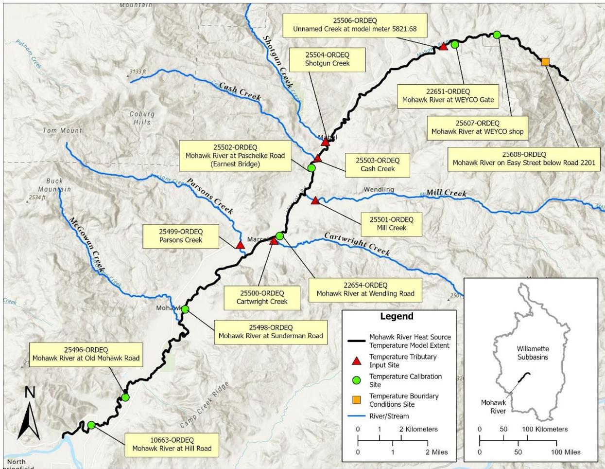
**Figure 3-181: Temperature monitoring locations used for the Mohawk River model setup and calibration.**
