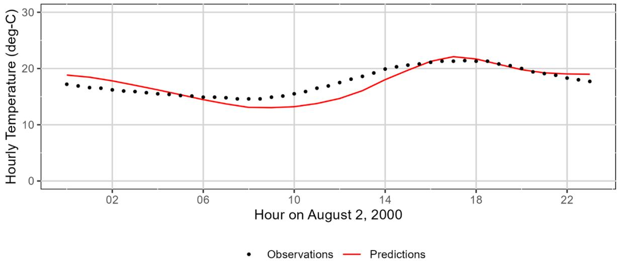
Figure 3-150: Crabtree Creek measured and model-predicted hourly temperatures at monitoring station 23743-ORDEQ.
