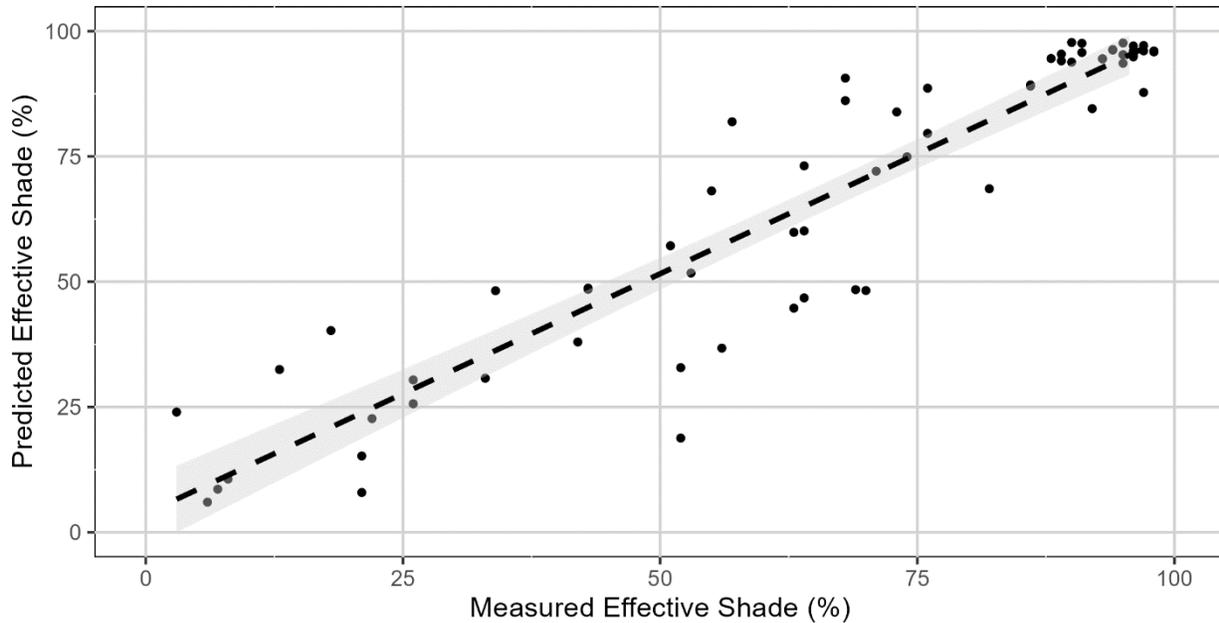
**Figure 3-249: Southern Willamette measured and predicted effective shade. The dashed line is the best fit line, and the grey area represents the confidence interval.**
