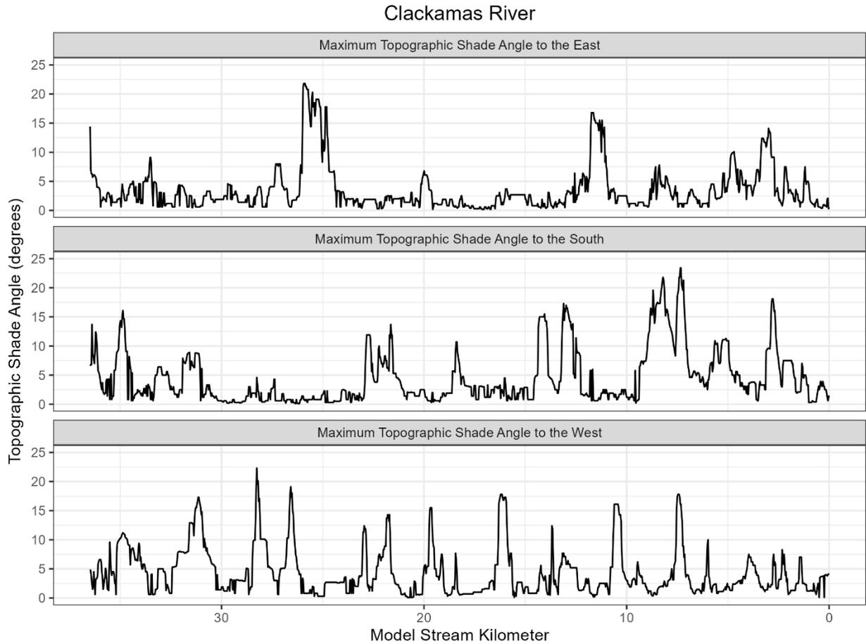
**Figure 3-263: Topographic shade angle inputs to the Clackamas River effective shade model.**
