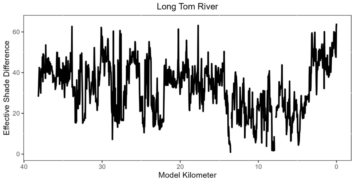
**Figure 4-95: Percentage point difference between effective shade from the Current Condition and Restored Vegetation scenarios on 8/1/2001 for the Long Tom River. Missing values indicate that the shade difference is negative due to instances of higher effective shade in the Current Condition scenario versus the Restored Vegetation scenario.**
