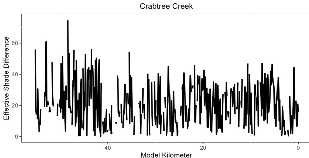
**Figure 4-62: Percentage point difference between effective shade from the Current Condition and Restored Vegetation scenarios on 8/2/2000 for Crabtree Creek. Missing values indicate that the shade difference is negative due to instances of higher effective shade in the Current Condition scenario versus the Restored Vegetation scenario.**
