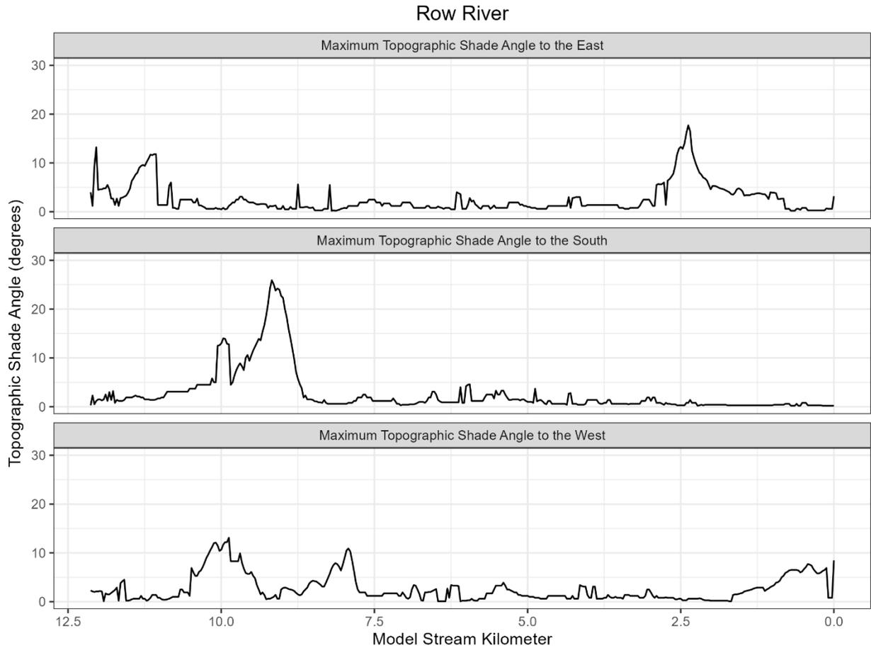
**Figure 3-275: Topographic shade angle inputs to the Row River effective shade model.**
