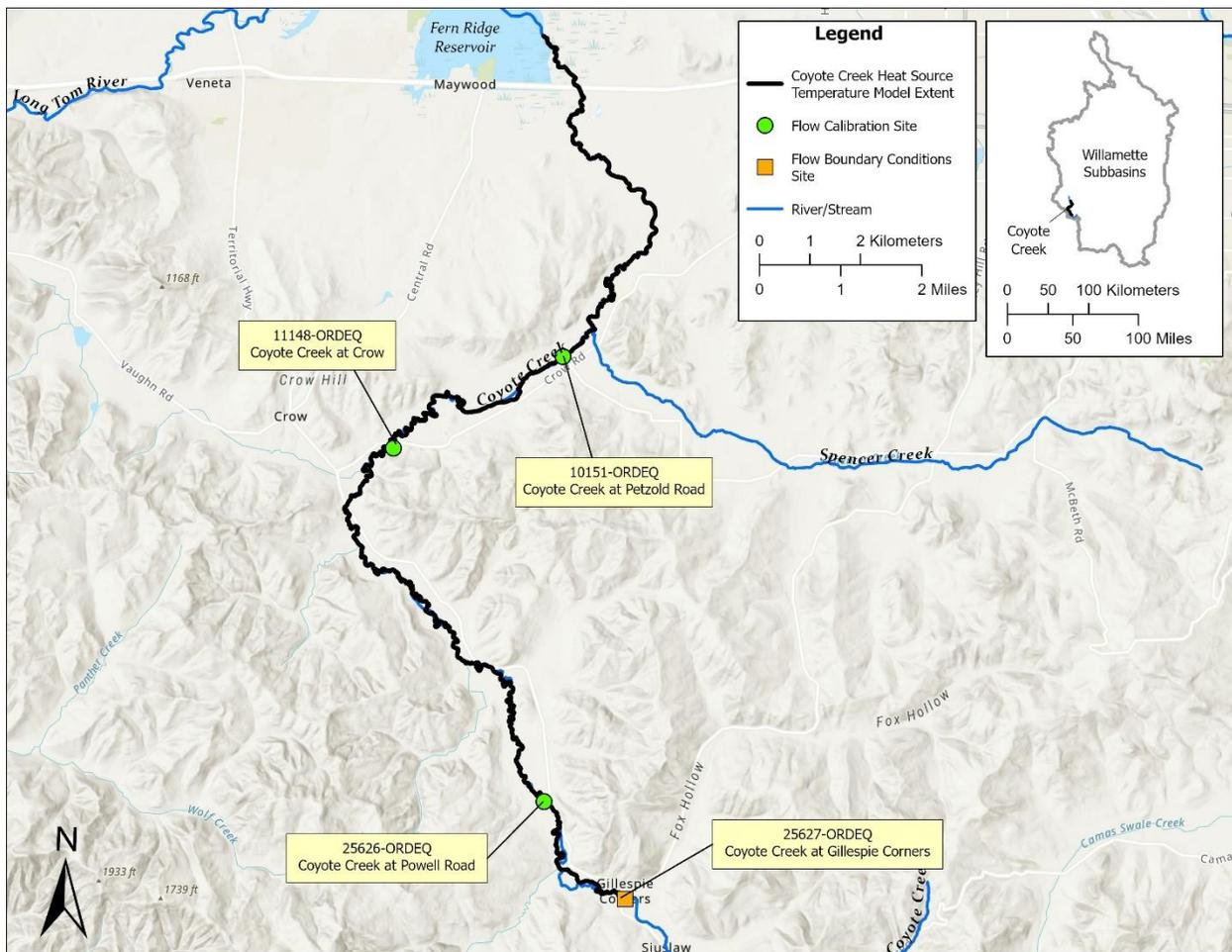
**Figure 3-217: Flow monitoring locations used for the Coyote Creek model setup and calibration.**
