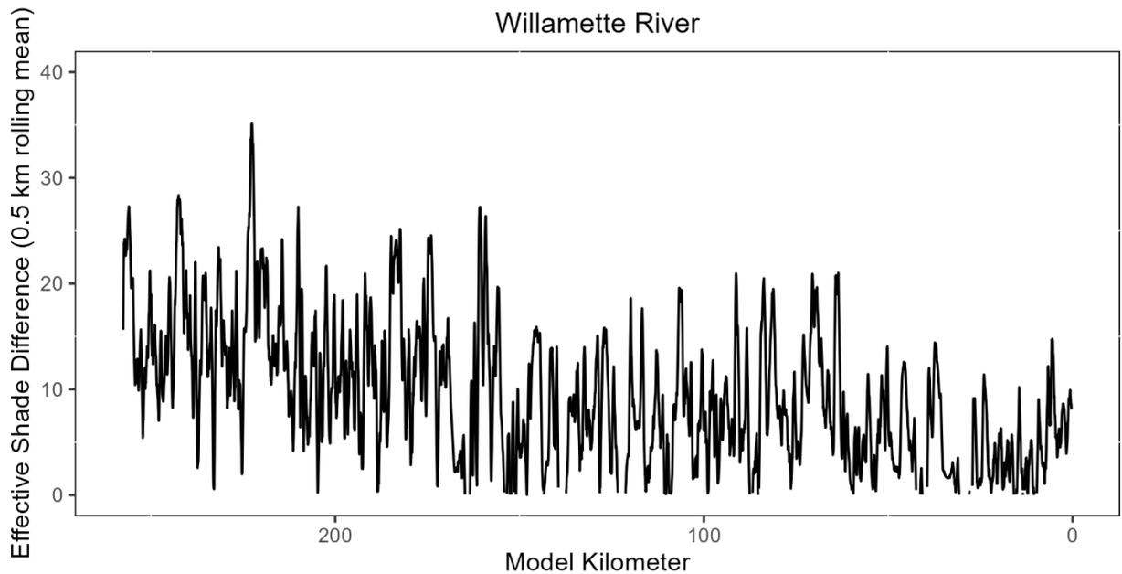
**Figure 4-87: Percentage point difference between half kilometer rolling mean effective shade from the Current Condition and Restored Vegetation scenarios on 8/1/2001 for the Willamette River. Missing values indicate that the shade difference is negative due to instances of higher effective shade in the Current Condition scenario versus the Restored Vegetation scenario.**
