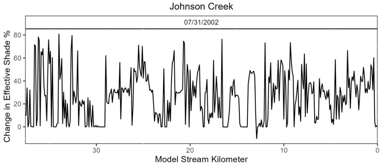
**Figure 4-4: Percentage point difference between effective shade from the Current Condition and Restored Vegetation scenarios on 7/31/2002 for Johnson Creek. Missing values indicate that the shade difference is negative due to instances of higher effective shade in the Current Condition scenario versus the Restored Vegetation scenario.**
