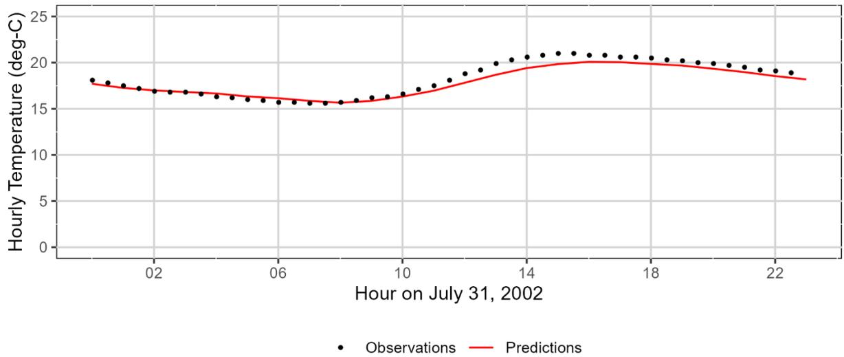
**Figure 3-10: Johnson Creek measured and model-predicted hourly temperatures at monitoring station 11321-ORDEQ.**
