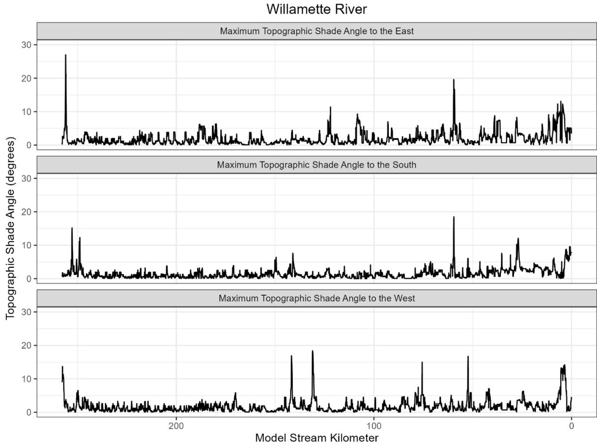
**Figure 3-261: Topographic shade angle inputs to the Willamette River effective shade model.**
