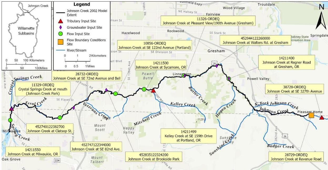
**Figure 3-5: Flow monitoring locations used for the Johnson Creek model setup and calibration.** The boundary condition and tributary flow inputs to the model is summarized in Table 3-4.
