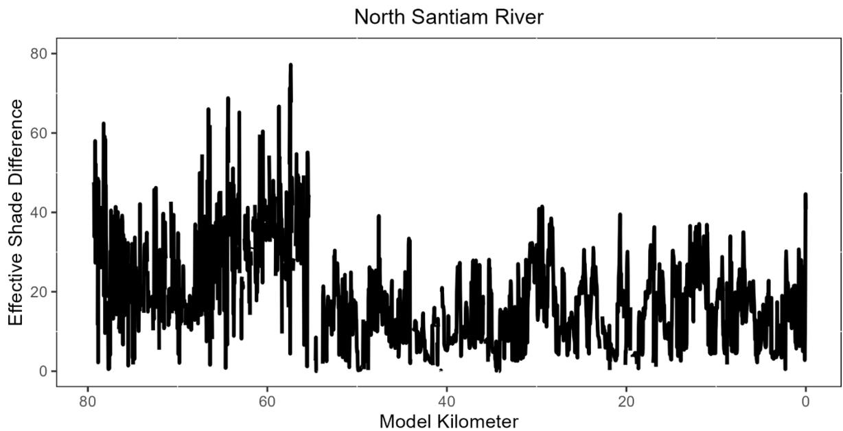
**Figure 4-99: Percentage point difference between effective shade from the Current Condition and Restored Vegetation scenarios on 8/1/2001 for the North Santiam River. Missing values indicate that the shade difference is negative due to instances of higher effective shade in the Current Condition scenario versus the Restored Vegetation scenario.**
