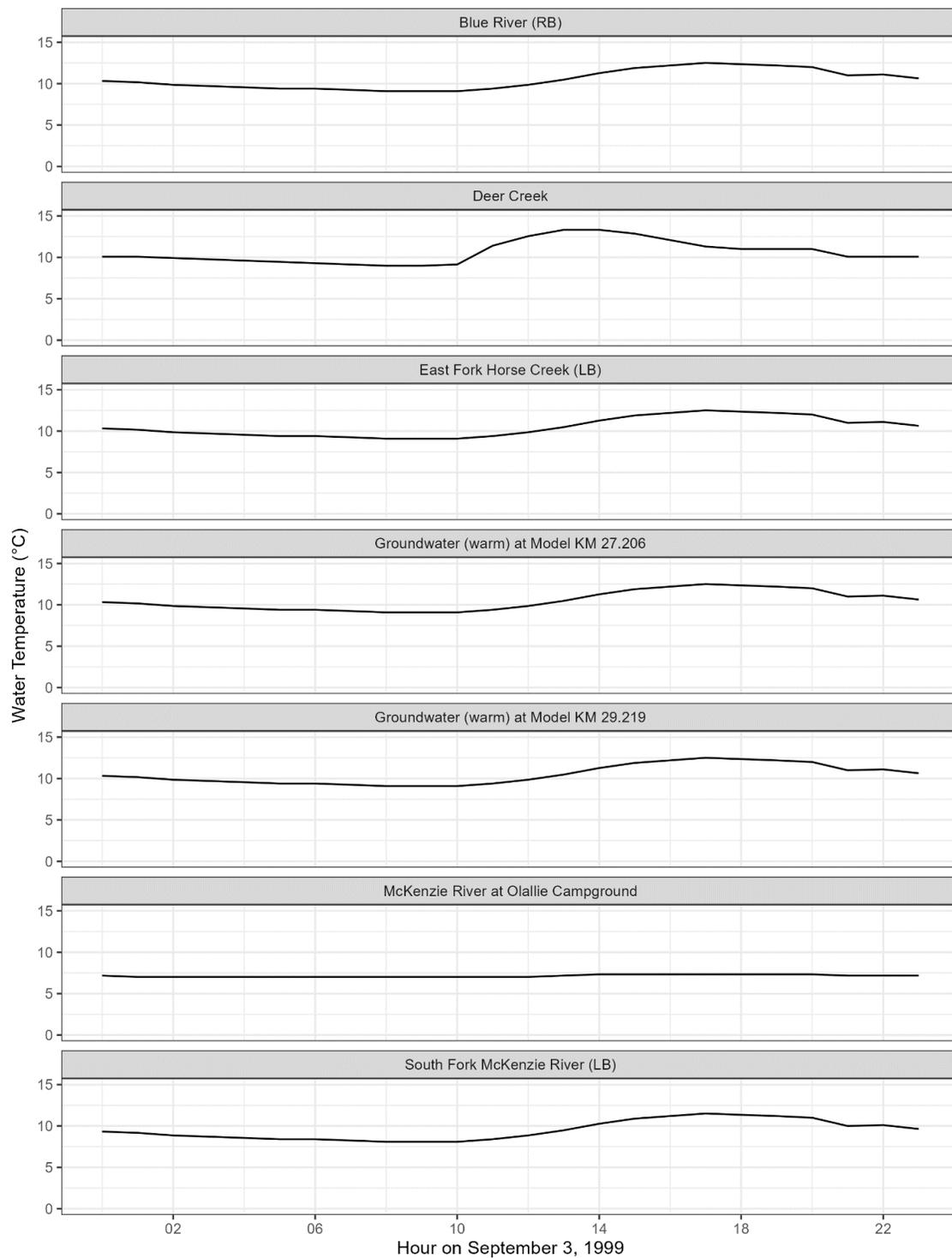
**Figure 3-201: Boundary condition, ground water and tributary water temperature inputs to the upper McKenzie River model.**
