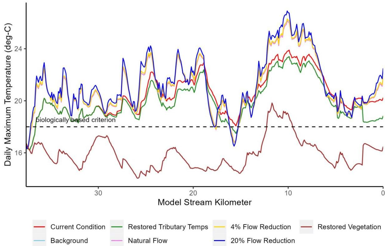
**Figure 4-1: Daily maximum stream temperature for all model scenarios for Johnson Creek. The temperature profile of the Background scenario exactly matches the Restored Vegetation scenario and is therefore not visible on the plot.**
