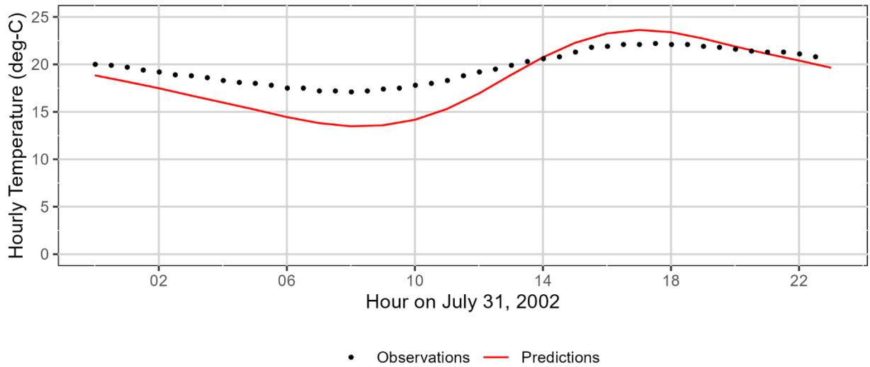
**Figure 3-14: Johnson Creek measured and model-predicted hourly temperatures at monitoring station 10853-ORDEQ.**
