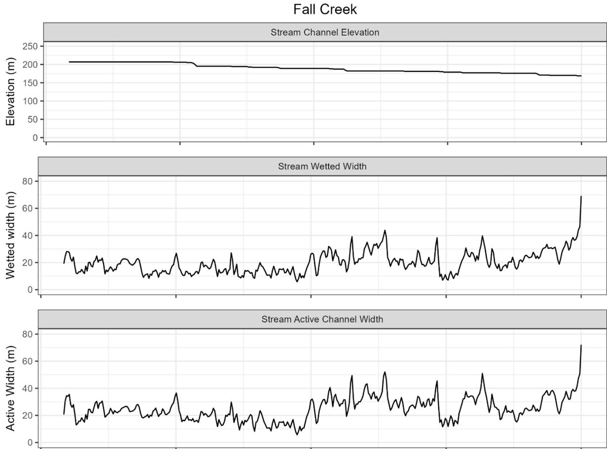
**Figure 3-283: Channel setup in the Fall Creek model.**
