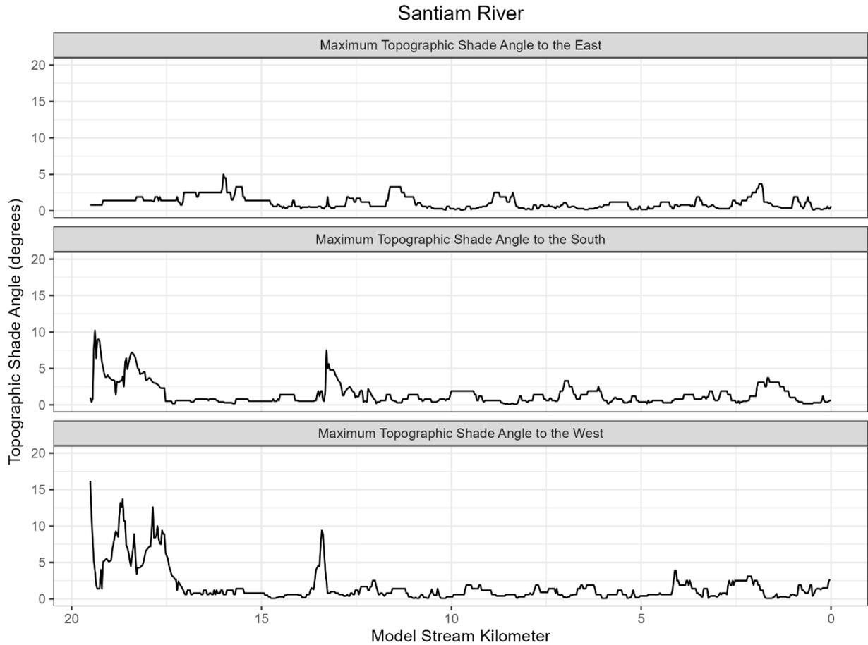
**Figure 3-277: Topographic shade angle inputs to the Santiam River effective shade model.**
