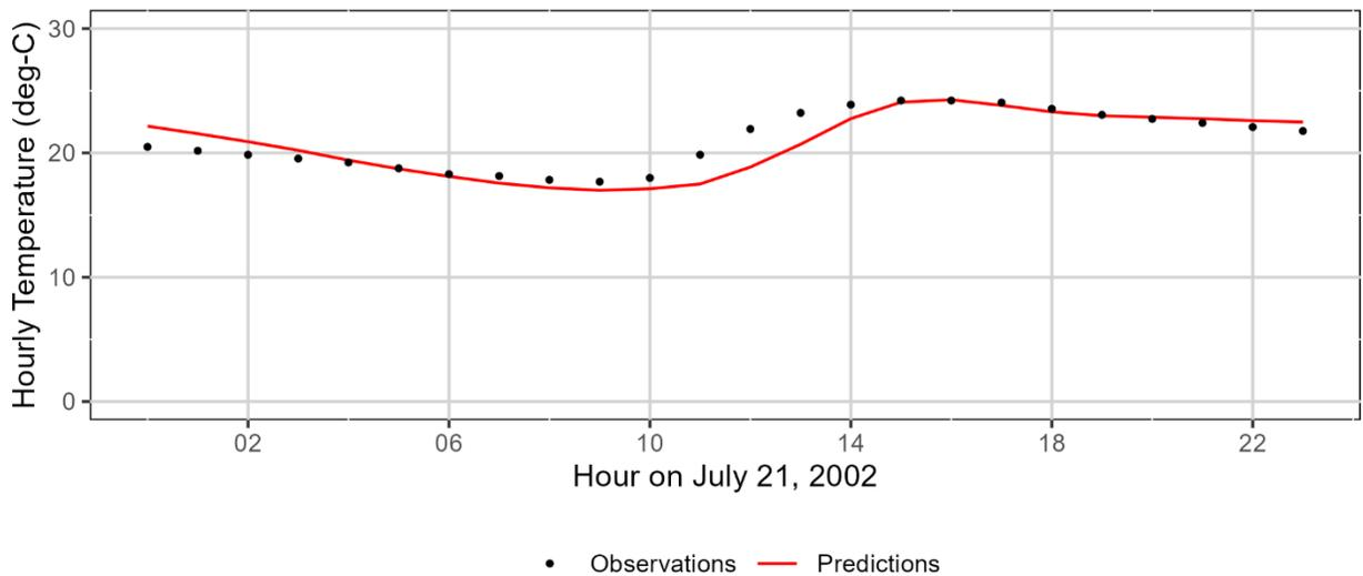
Figure 3-240: Mosby Creek measured and model-predicted hourly temperatures at monitoring station 28799-ORDEQ.
