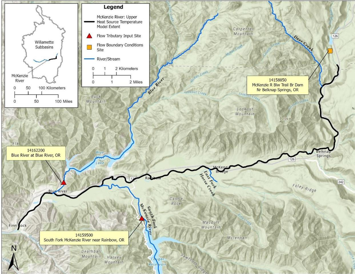
**Figure 3-202: Flow monitoring locations used for the upper McKenzie River model setup and calibration.**
