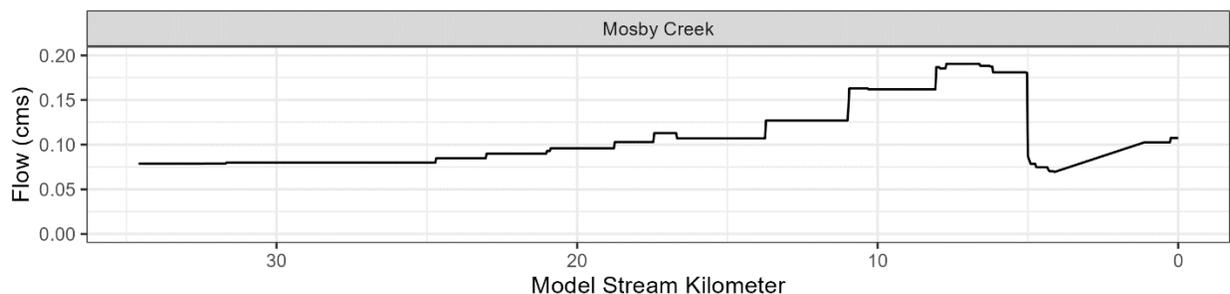
**Figure 3-234: Boundary condition and mainstem flow inputs to the Mosby Creek model.**
