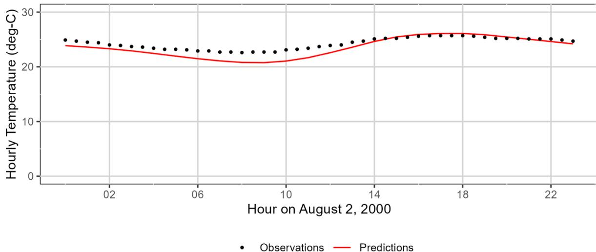
**Figure 3-144: Crabtree Creek measured and model-predicted hourly temperatures at monitoring station 10784-ORDEQ.**
