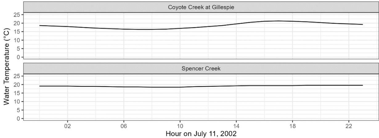
Figure 3-216: Boundary condition and tributary water temperature inputs to the Coyote Creek model.
