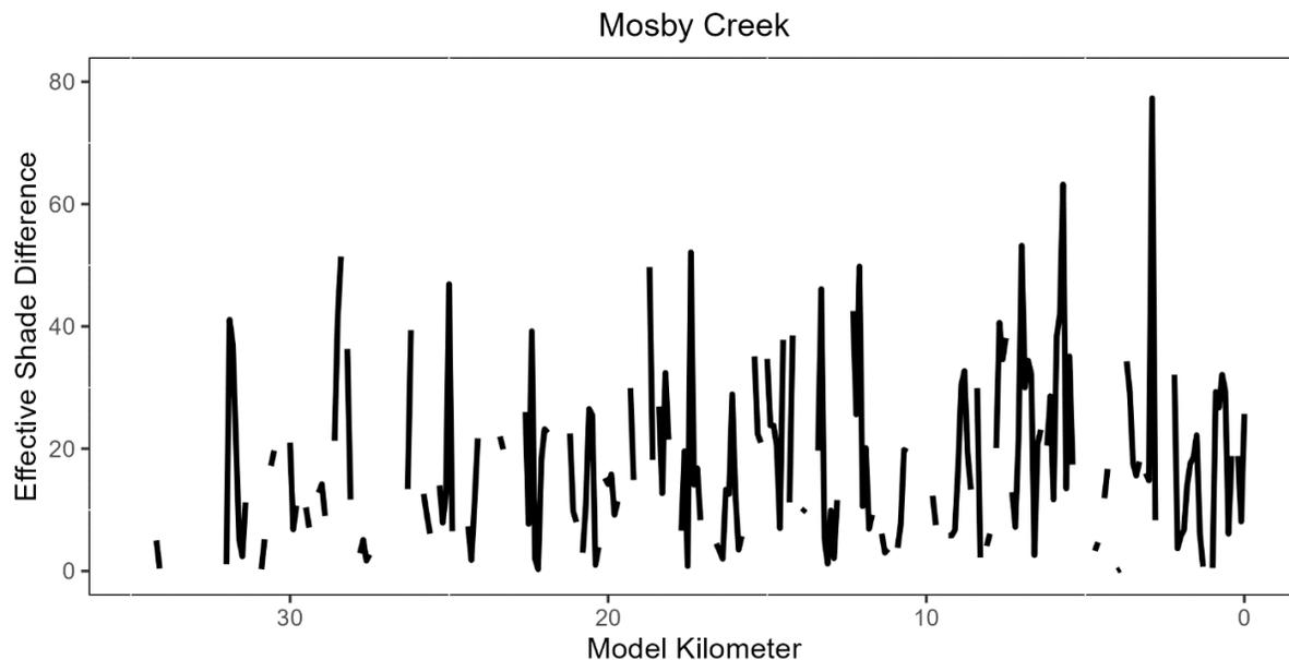
**Figure 4-83: Percentage point difference between effective shade from the Current Condition and Restored Vegetation scenarios on 7/21/2002 for Mosby Creek. Missing values indicate that the shade difference is negative due to instances of higher effective shade in the Current Condition scenario versus the Restored Vegetation scenario.**
