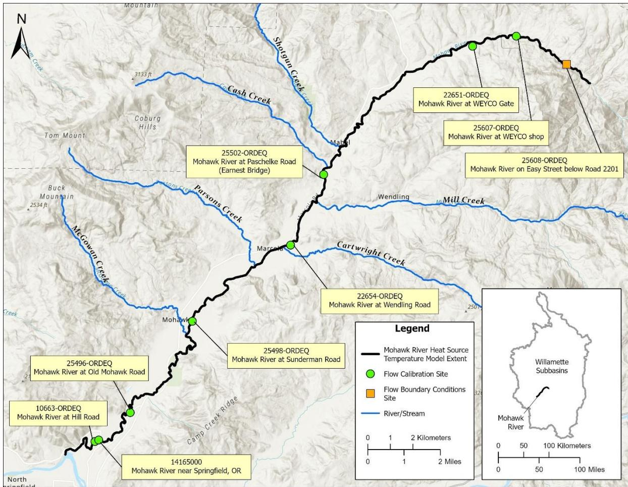
**Figure 3-183: Flow monitoring locations used for the Mohawk River model setup and calibration.**
