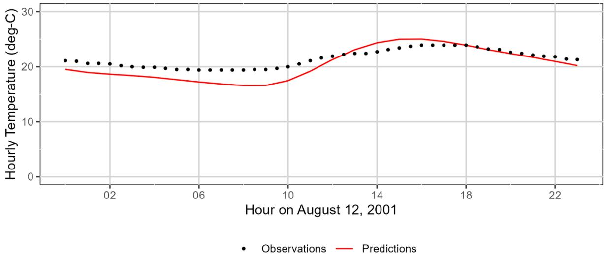
**Figure 3-169: Luckiamute River measured and model-predicted hourly temperatures at monitoring station 25483-ORDEQ.**
