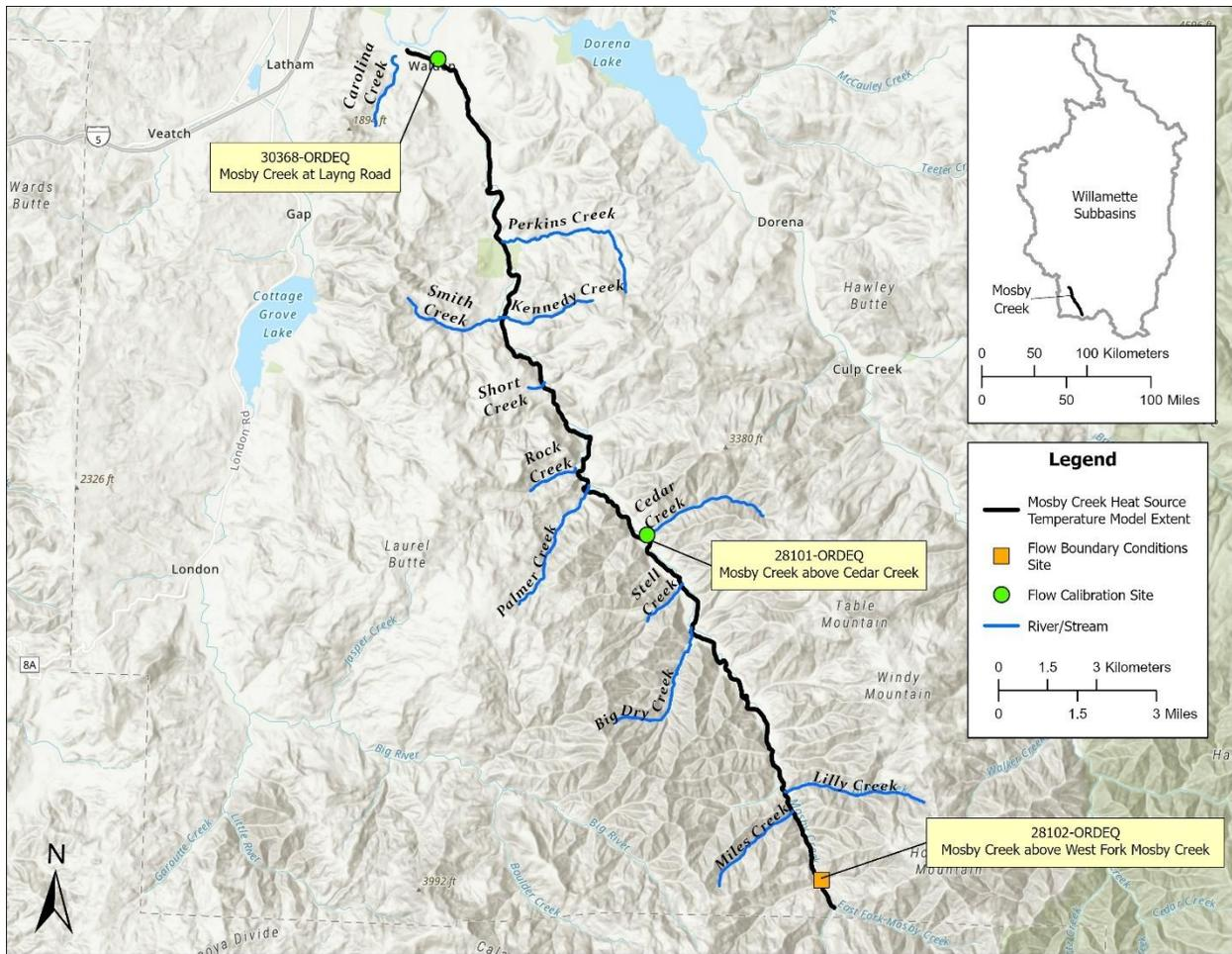
**Figure 3-233: Flow monitoring locations used for the Mosby Creek model setup and calibration.**
