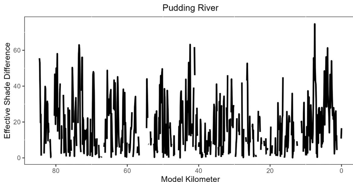
**Figure 4-25: Percentage point difference between effective shade from the Current Condition and Restored Vegetation scenarios for the Pudding River. Missing values indicate that the shade difference is negative due to instances of higher effective shade in the current condition scenario versus the restored vegetation scenario.**
