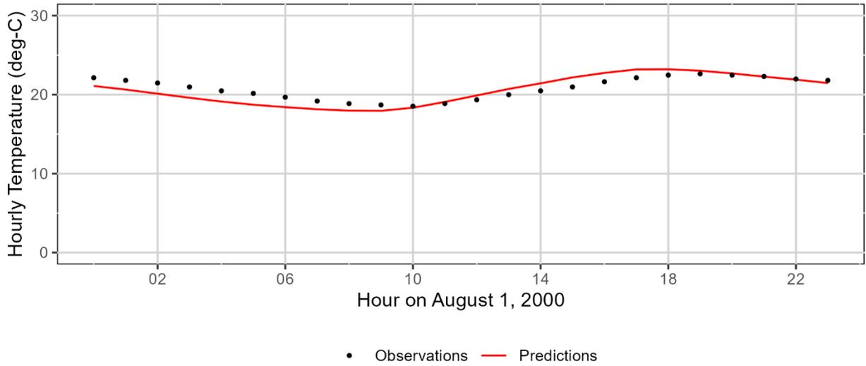
**Figure 3-107: Little North Santiam River measured and model-predicted hourly temperatures at monitoring station S349766.**
