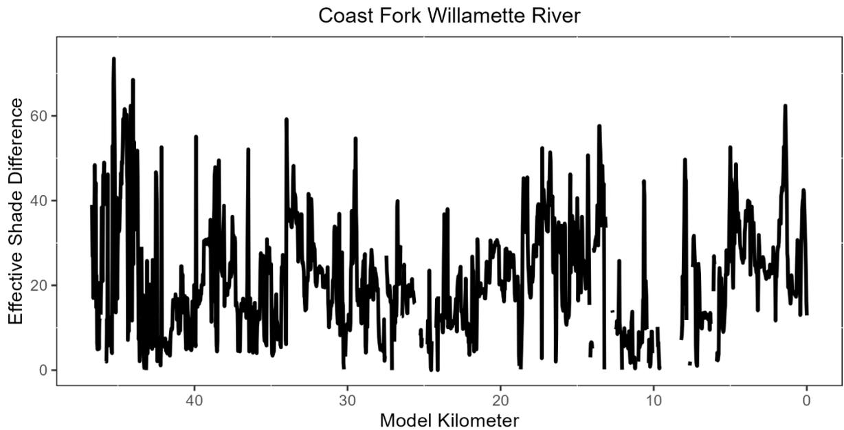
**Figure 4-91: Percentage point difference between effective shade from the Current Condition and Restored Vegetation scenarios on 8/1/2001 for the Coast Fork Willamette River. Missing values indicate that the shade difference is negative due to instances of higher effective shade in the Current Condition scenario versus the Restored Vegetation scenario.**
