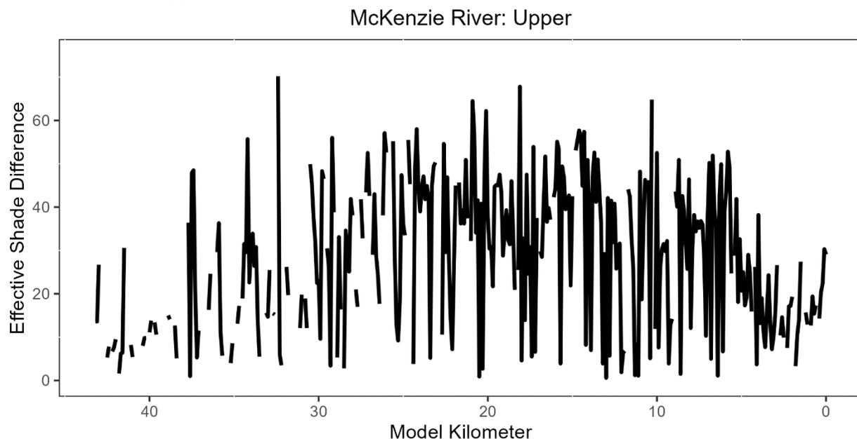
**Figure 4-74: Percentage point difference between effective shade from the Current Condition and Restored Vegetation scenarios on 9/3/1999 for the upper McKenzie River. Missing values indicate that the shade difference is negative due to instances of higher effective shade in the Current Condition scenario versus the Restored Vegetation scenario.**
