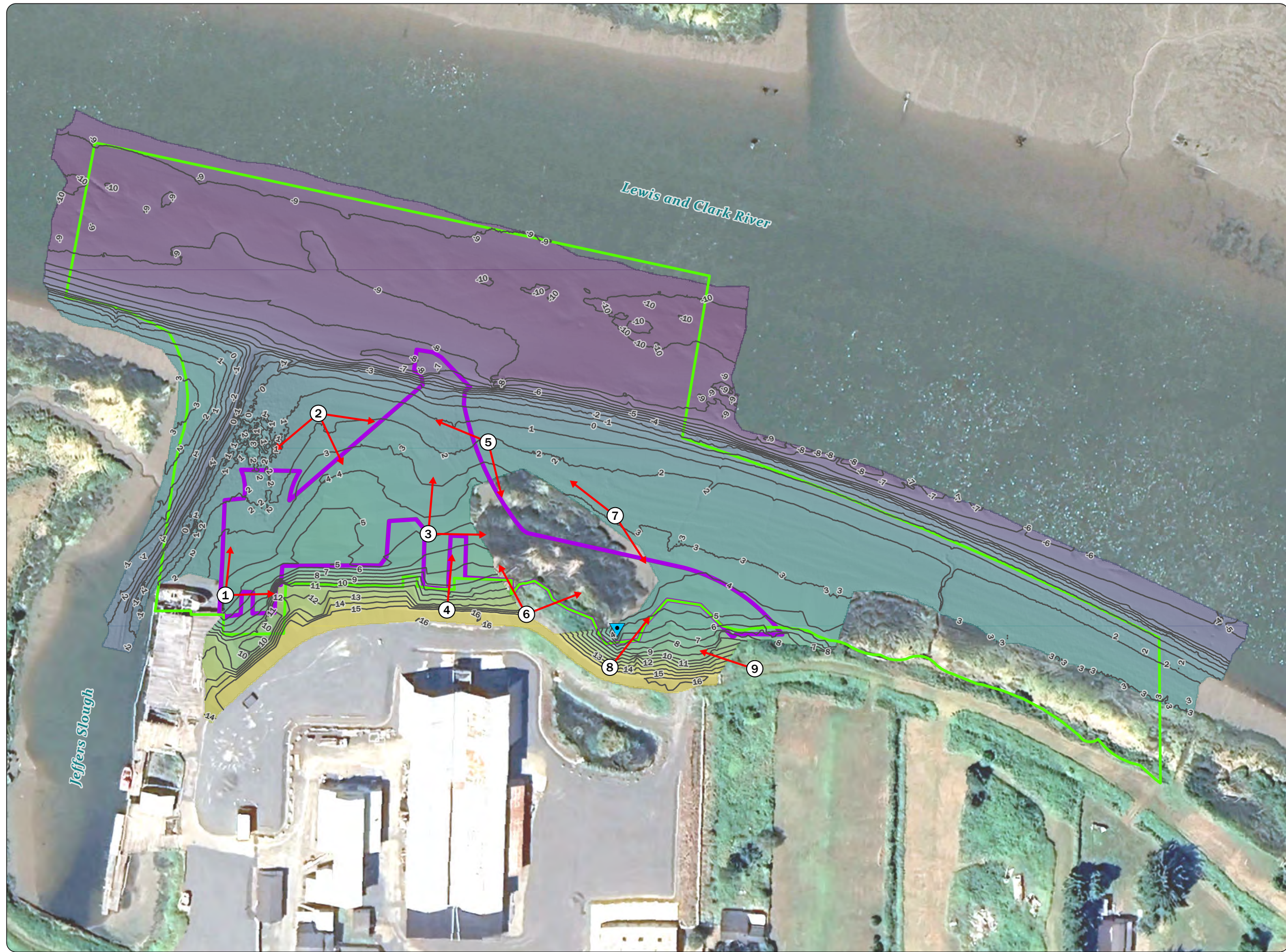
Figure 3-1 Photograph Locations for Visual Monitoring and 2024 Bathymetric Survey Results
