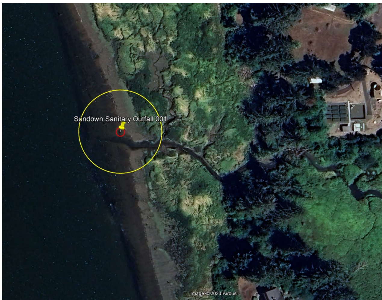
Figure 3-1: Outfall 001 with original ZID (red circle) and RMZ (yellow circle)
