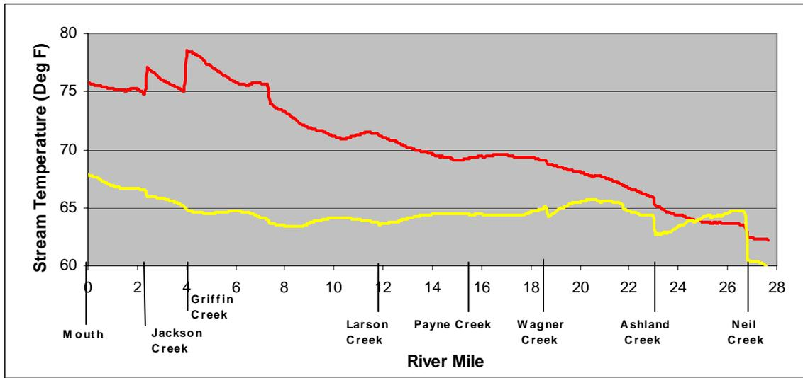
Note: Red line is current conditions stream temperatures, yellow line is predicted temperature profile under the natural thermal potential scenario.
