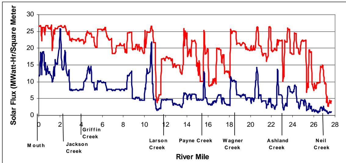
Note: red line is current conditions thermal load, blue line is predicted thermal load under a natural thermal potential scenario.
