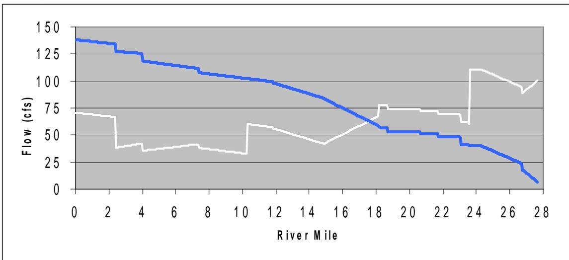
Note: Current Conditions (white line) as measured August 3, 1999. Blue line predicted flow under natural conditions. Source USBOR and DEQ. See Appendix A for a more complete discussion of thermal modeling and flow.
