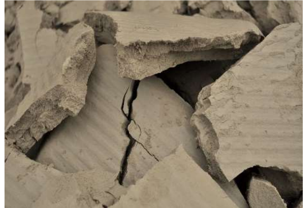
Chemical etching and milling filter cake from dewatered sludge. Photo D. Lobato
