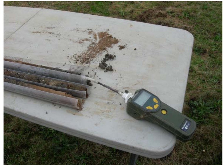
Using a PID to determine if soils are impacted with volatile organics.
