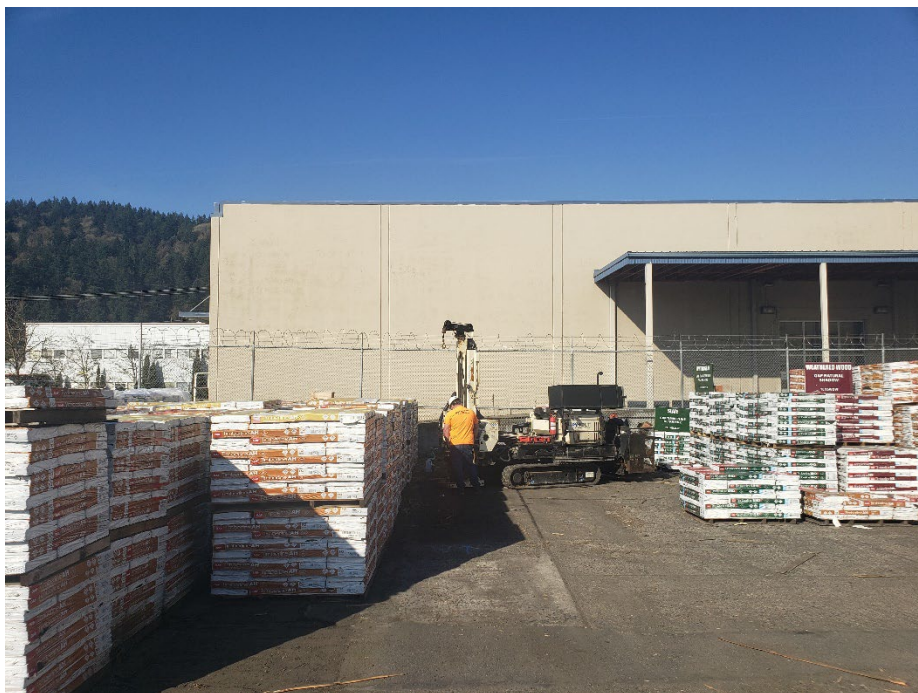
Photo 1. Collecting soil gas sample SV-3 adjacent to the western property boundary with a post-run tubing (PRT) sampling system.
