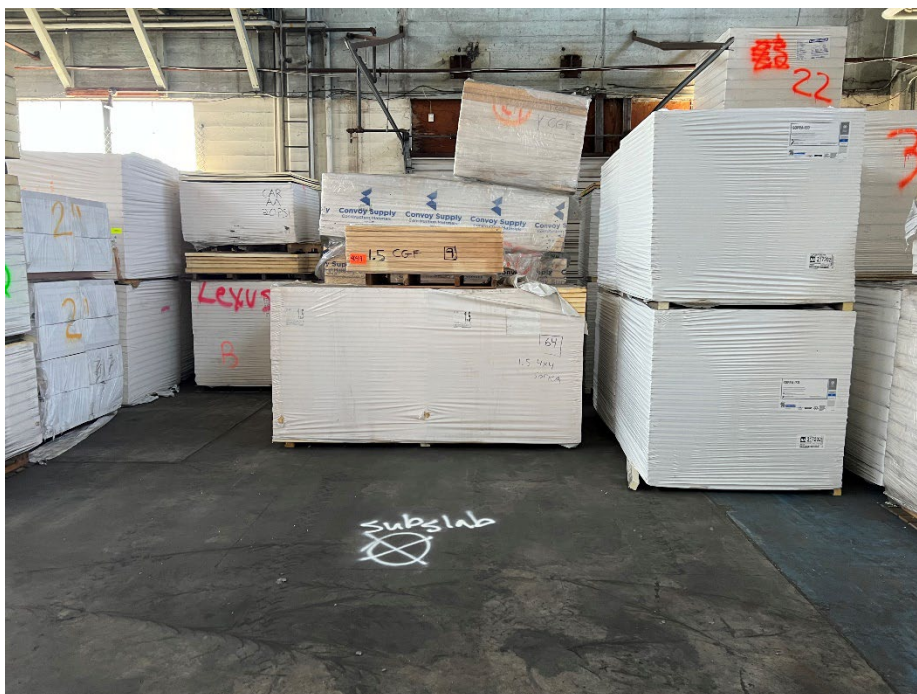
Photo 4. Sub-slab sample location SSV-2 marked out in paint near the southern end of the warehouse.
