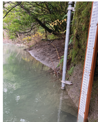
Staff plate and crest gage installed in Pistol River.
