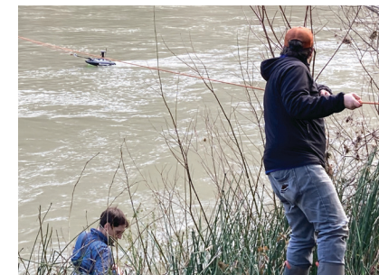
Contractors deploy an Acoustic Doppler Coupled Profiler to measure discharge during a moderately high flow in Pistol River (~4,000 cfs).
