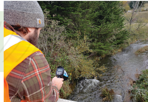
Robbie Lascheck uses a specialized radar gun to measure the velocity of a stream from the safety of a bridge.
