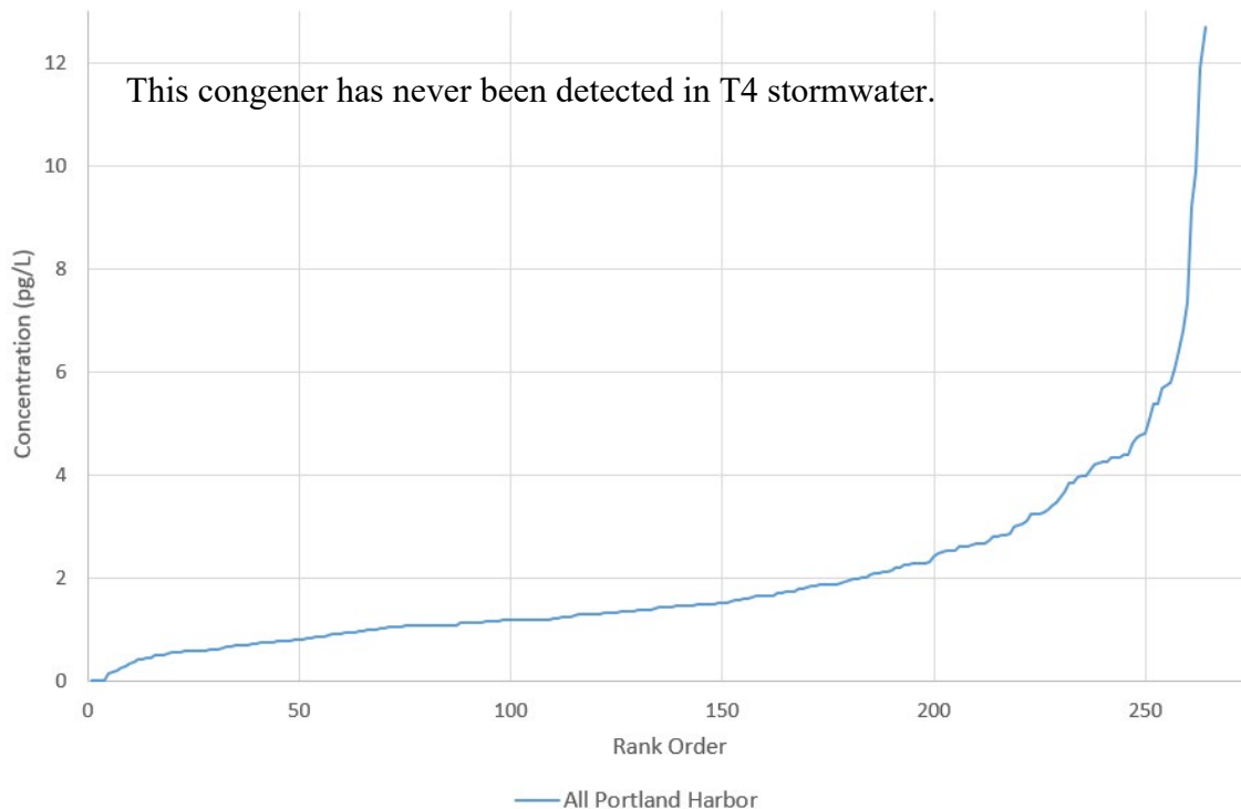
Figure B - 26. 1,2,3,7,8,9-HxCDF in Stormwater at T4 Compared to “Typical” Industrial Stormwater in the Portland Harbor
