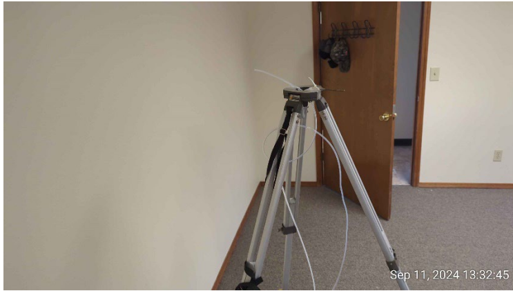
View of intake tubing at top of tripod
