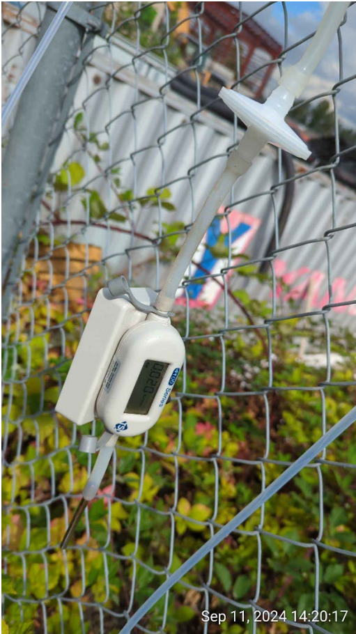
EPA Method TO-17 intake location for outdoor air sample. View of digital flow meter during sample setup.
