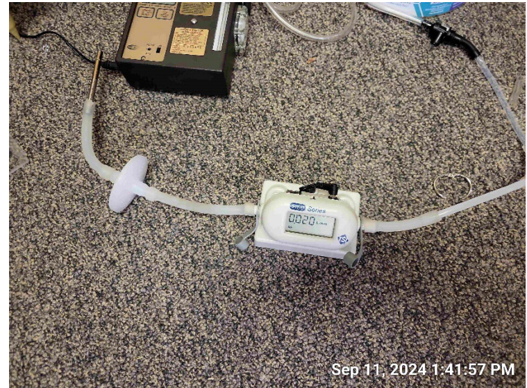
Calibrating flow rate for EPA Method TO-17 sample using digital flow meter.
