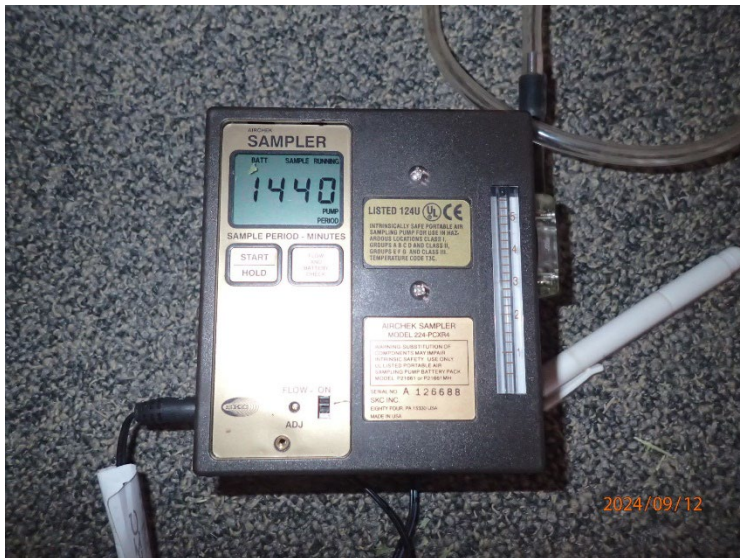
TO-17 samples were collected after 24-hours (1440 minutes).
