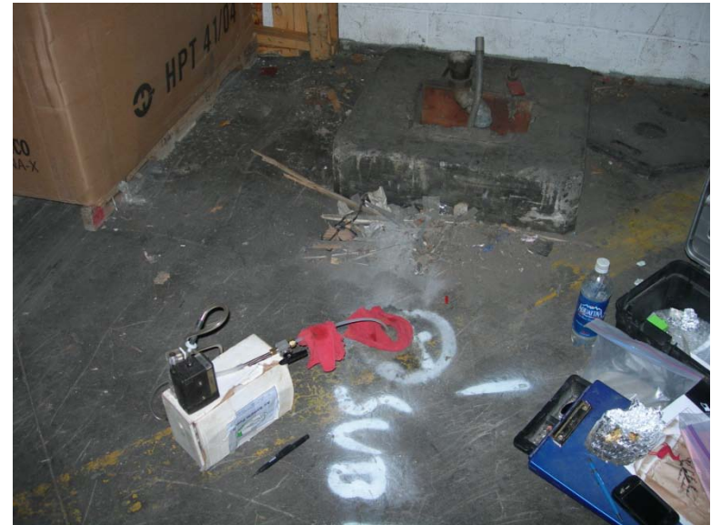
Collecting sub-slab vapor sample SUB01.
