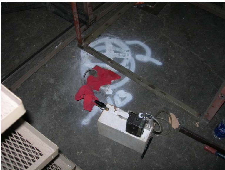
Collecting sub-slab vapor sample. Red rags contain 2-propanol as a test for system leakage during sampling.
