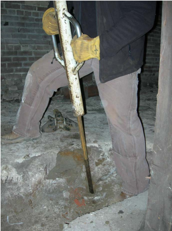
Manually advancing push probe to recover soil samples within the crawlspace of the building.
