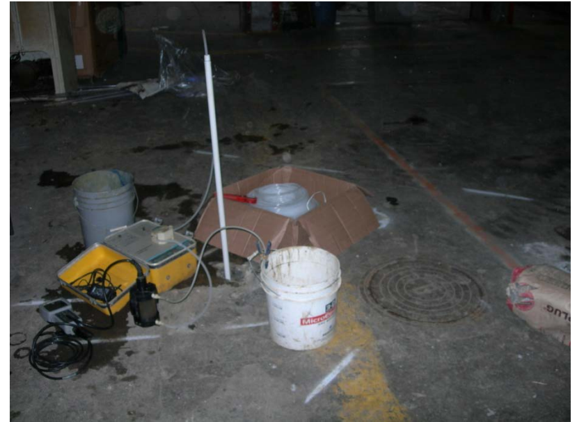
Collecting water sample from temporary well point in boring adjacent to dry well/cistern.
