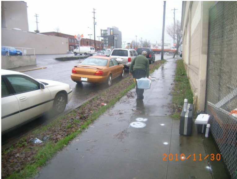
Geophysical survey in progress to clear for Phase II drilling locations.
