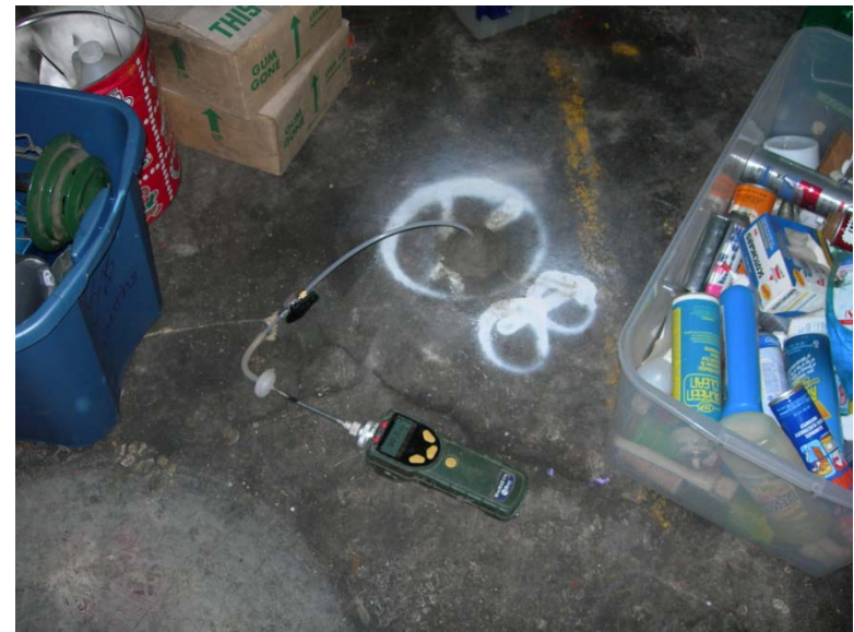
Screening sub-slab vapor sample location with a PID.
