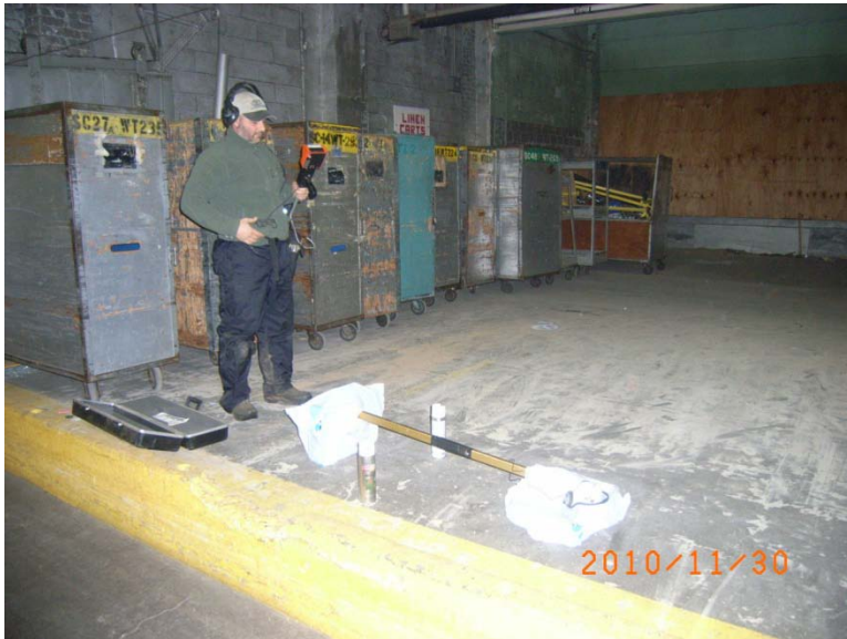
Geophysical survey within building to clear proposed boring locations.
