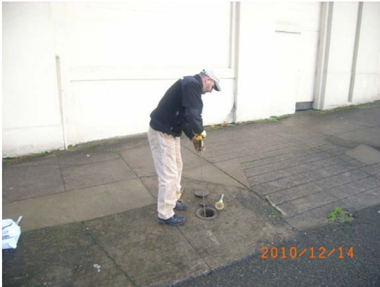
Checking tank contents and depth of abandoned tank on south side of property.
