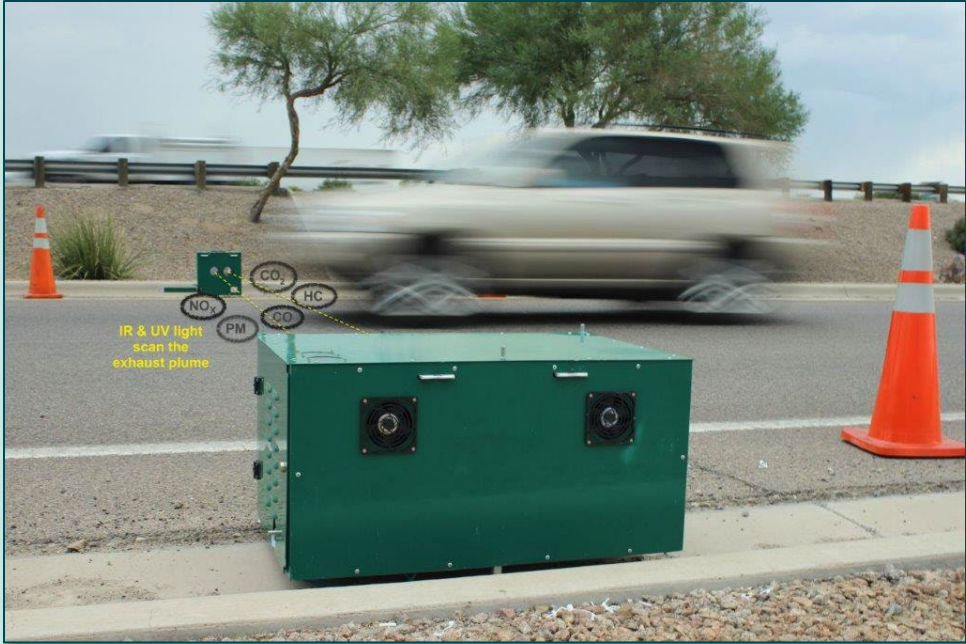
Figure 1: Unattended RSD5300 on-road deployment
