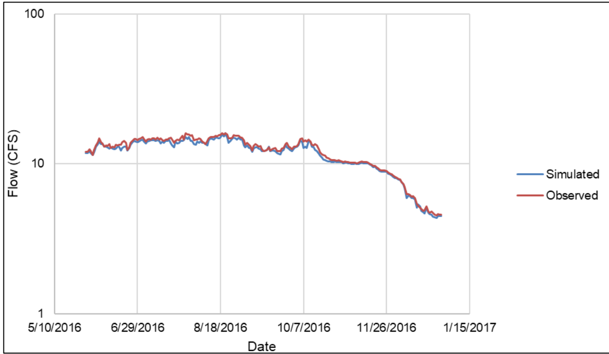
Figure 12. Observed and modeled mean daily flow rates at Bowman's Bridge (USGS 14140000), 2016 model calibration period
