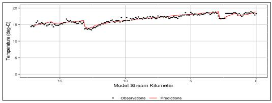
Figure 3-31: Little Sandy River longitudinal temperatures: Modeled vs. TIR-observed, 2pm 8/9/2001.
