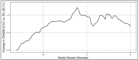
Figure 4-3: Salmon River scenario results: Longitudinal 7DADM temperature differences, CCC vs. RV\_B.
