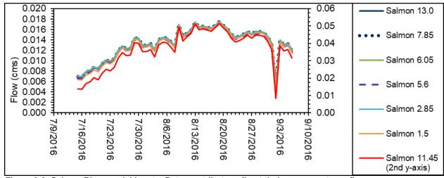
Figure 3-8: Salmon River model inputs: Between-tributary direct drainage area streamflows.
