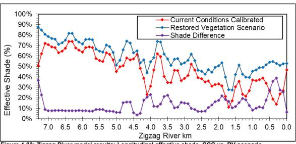
Figure 4-23: Zigzag River model results: Longitudinal effective shade, CCC vs. RV scenario.
