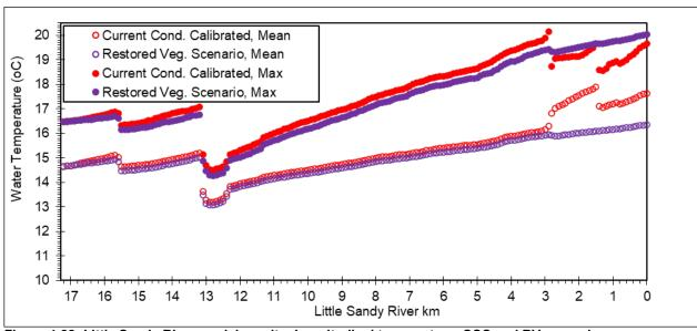
Figure 4-22: Little Sandy River model results: Longitudinal temperature, CCC and RV scenario.
