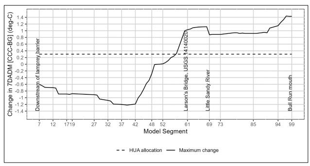
Figure 4-30: Bull Run R. model results: Longitudinal maximum 7DADM temperature, CCC minus BG scenario
