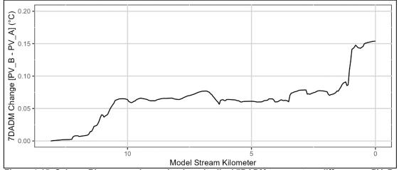
Figure 4-15: Salmon River scenario results: Longitudinal 7DADM temperature differences: PV\_B vs. PV\_A.
