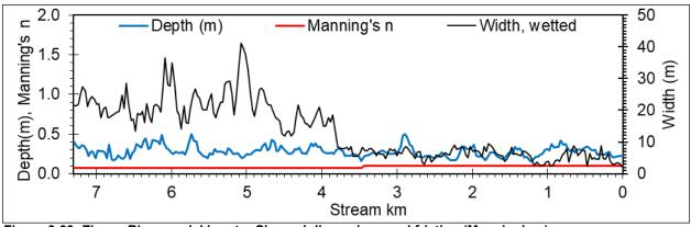
Figure 3-39: Zigzag River model inputs: Channel dimensions and friction (Manning's n).
