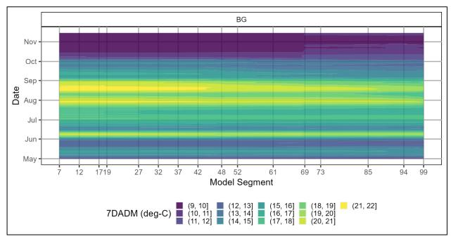
Figure 4-29: Bull Run River BG 7DADM temperatures by model segment and date.
