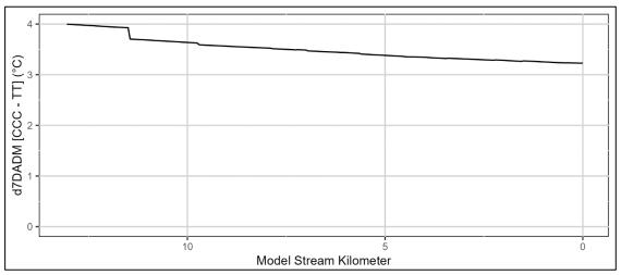
Figure 4-19: Salmon River scenario results: Longitudinal 7DADM temperature differences, TT vs. CCC.
