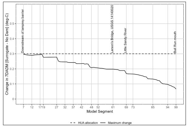
Figure 4-33: Bull Run River maximum 7DADM temperature changes above the applicable criteria due to Bull Run River dams and reservoirs with discharges attaining the surrogate measure.
