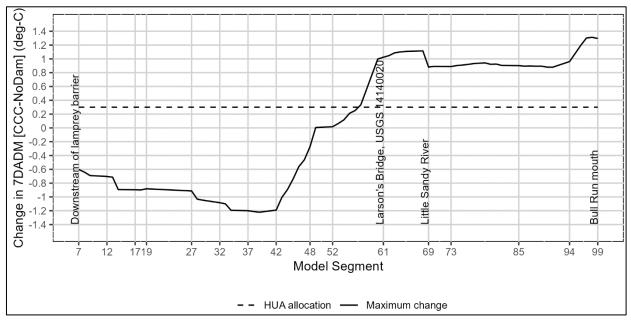
Figure 4-25: Bull Run River model results: Longitudinal maximum 7DADM temp differences, CCC minus No Dams.
