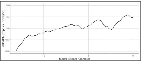
Figure 4-18: Salmon River scenario results: Longitudinal 7DADM temp differences, Topography vs. CCC.
