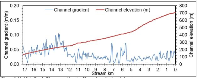
Figure 3-26: Little Sandy River model inputs: Channel gradient and elevation.
