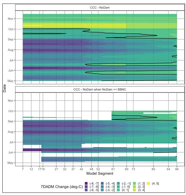
Figure 4-27: Bull Run River model results: 7DADM temp differences, CCC minus No Dams.
