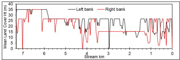
Figure 3-38: Zigzag River model inputs: Landcover height.
