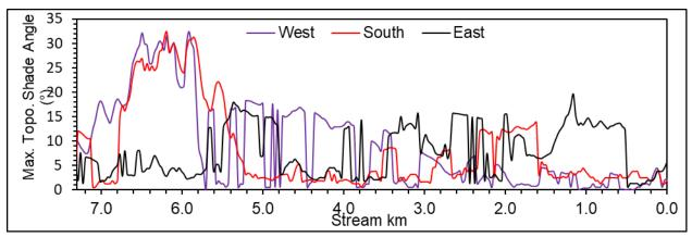
Figure 3-37: Zigzag River model inputs: Maximum topographic shade angles.
