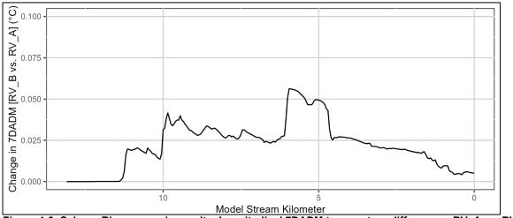
Figure 4-6: Salmon River scenario results: Longitudinal 7DADM temperature differences, RV\_A vs. RV\_B.
