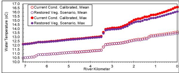
Figure 4-24: Zigzag River model results: Longitudinal temperature, CCC and RV scenario.
