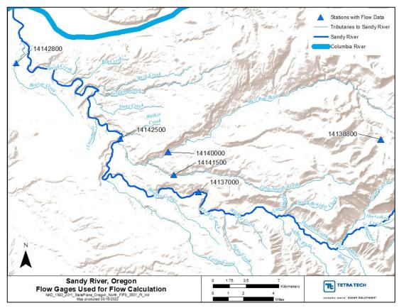
Figure 2-1: Sandy Subbasin streamflow measurement sites.
