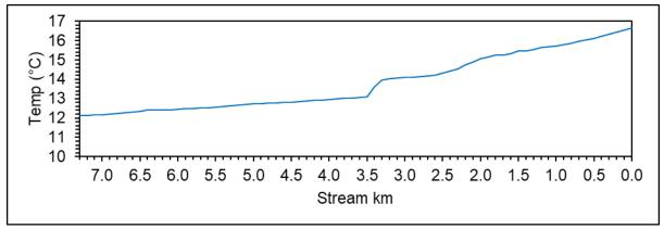
Figure 3-45: Zigzag River model results: Longitudinal daily maximum temperatures, 8/9/2001.
