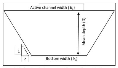
Figure 2-3: Equation 2-1 conceptual diagram: Trapezoidal channel and terms.
