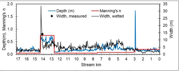
Figure 3-27: Little Sandy River model inputs: Channel dimension and friction (Manning's n).
