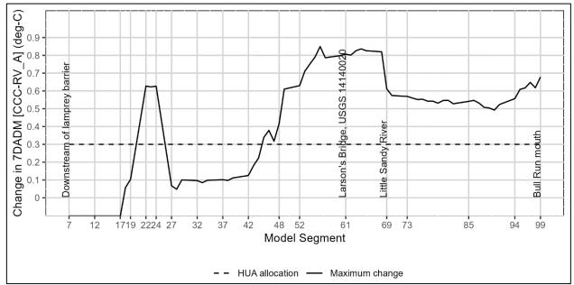
Figure 4-28: Bull Run River model results: Longitudinal maximum 7DADM temperature differences, CCC vs. RV\_A.
