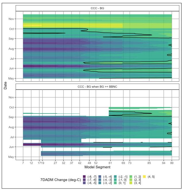
Figure 4-32: Bull Run River model results: 7DADM temperature differences, CCC minus BG by model segment and date.
