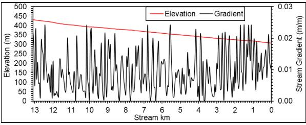
Figure 3-13: Salmon River model inputs: Stream channel elevation and gradient.
