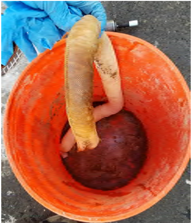
SORBENT SOCK INSTALLED IN MONITORING WELL MW-8. PHOTOGRAPH TAKEN MAY 4, 2021.
