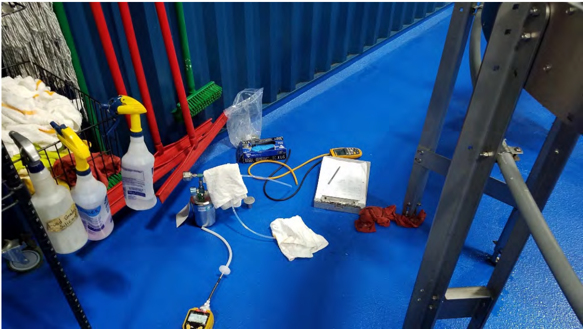
SUB-SLAB VAPOR SAMPLING. PHOTOGRAPH TAKEN AUGUST 11, 2021.
