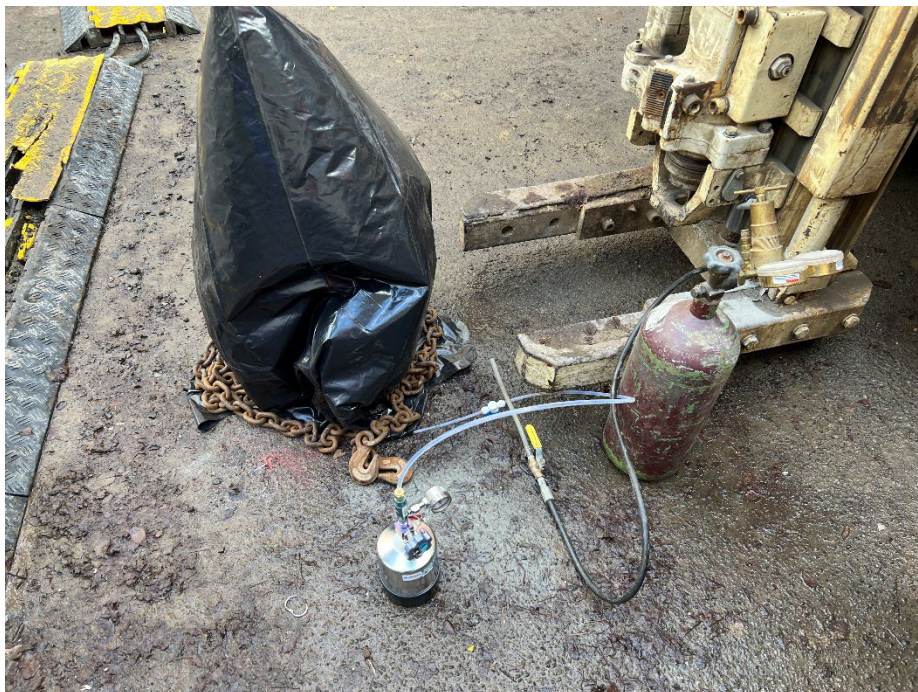
Photo 6. A soil gas sample was collected from boring B-6 using a post-run tubing (PRT) sampler. Helium was used as a tracer gas for leak detection.
