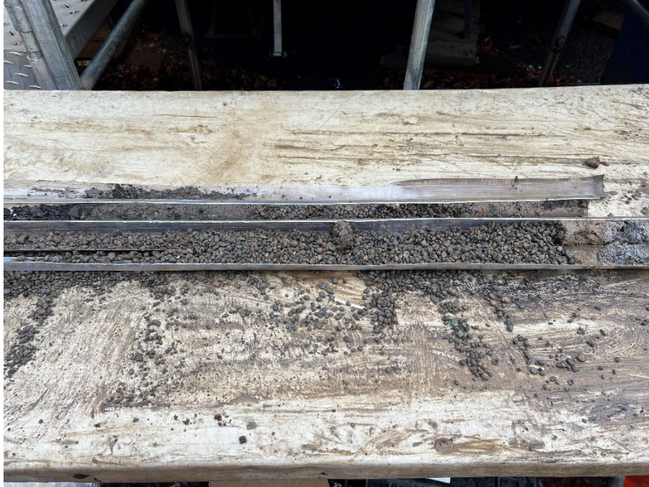
Photo 5. Pea gravel backfill material was observed in borings B-1 and B-3, advanced through the large excavation that was detected during the geophysical survey.
