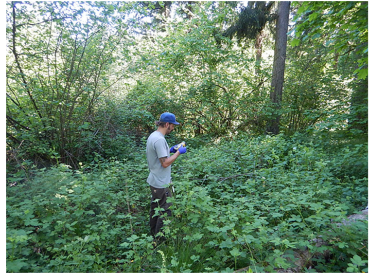
Import Soil Characterization - each subsample location was recorded using a handheld GPS unit. This assured obtaining 64 subsamples across the site with appropriate coverage.
