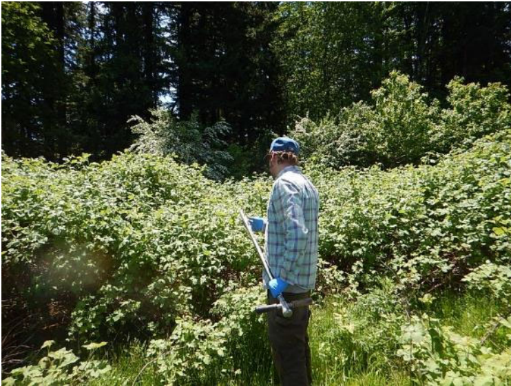
Import Soil Characterization - soil samples were obtained using a stainless-steel probe, advanced approximately 6-inches bgs, with the lower 3 to 4 inches retained.
