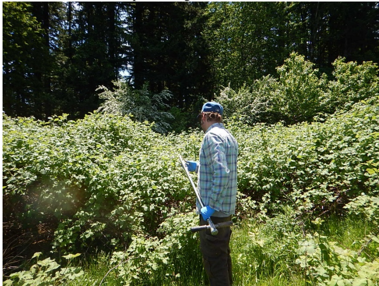
Soil samples were obtained using a stainless-steel probe, advanced approximately 6-inches BGS, with the lower 3 to 4 inches sampled.
