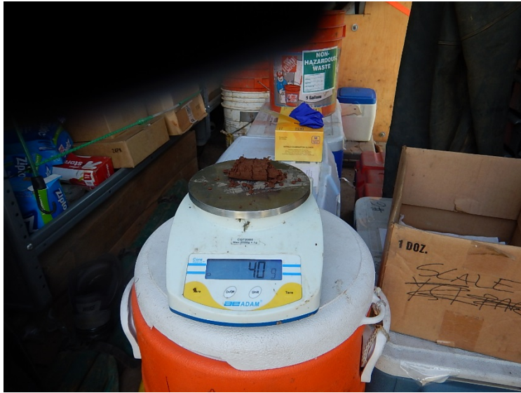
An approximate 40-gram core is obtained from each subsample location. These are collected in a dedicated 1-gallon jar and submitted to the lab for processing.
