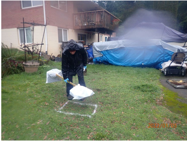
Geophysical survey of south residence (10400 SE Vradenburg) located a possible old septic tank (MA01).
