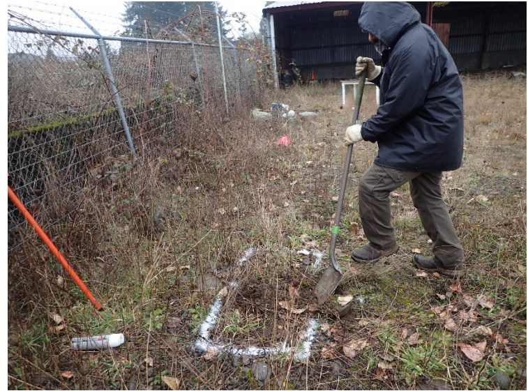
Magnetic anomalies marked in white paint were later exhumed to determine their source. No buried USTs were identified.
