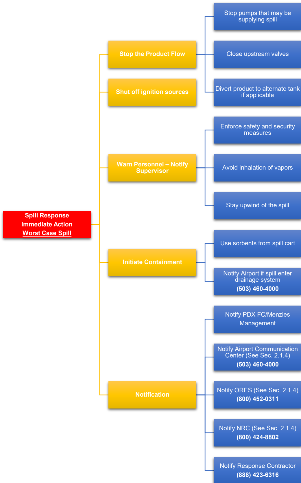
Figure 2-5: Spill Response, Worst Case Spill
