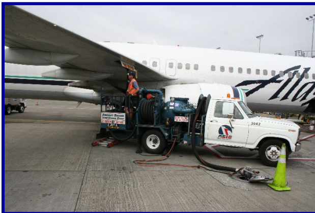
Hydrant servicer fueling aircraft.
