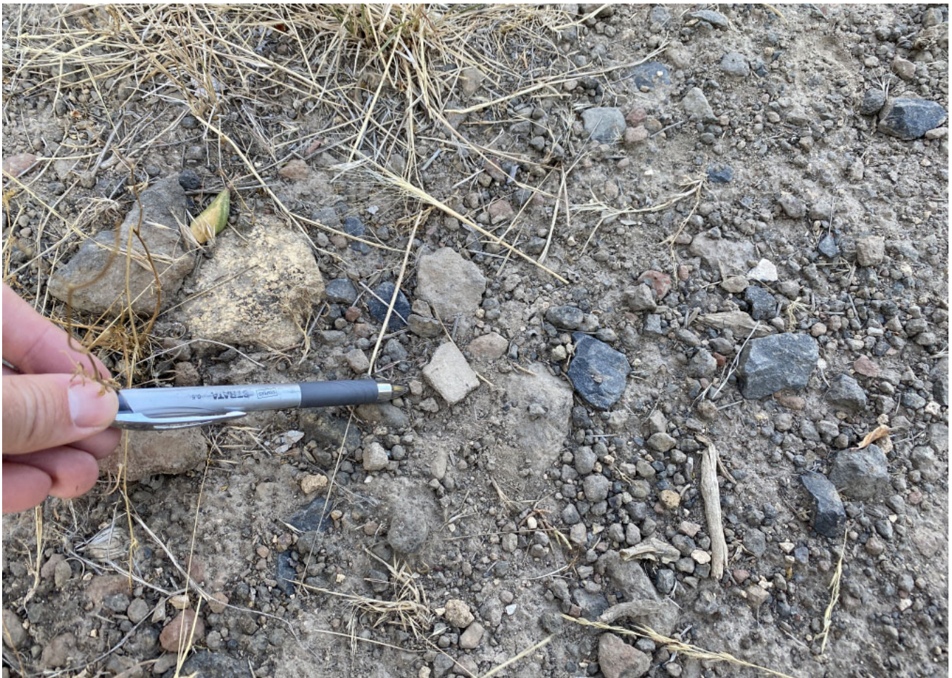
One piece of concrete asbestos board (CAB) was located during inspection. It was approximately 1" square.
